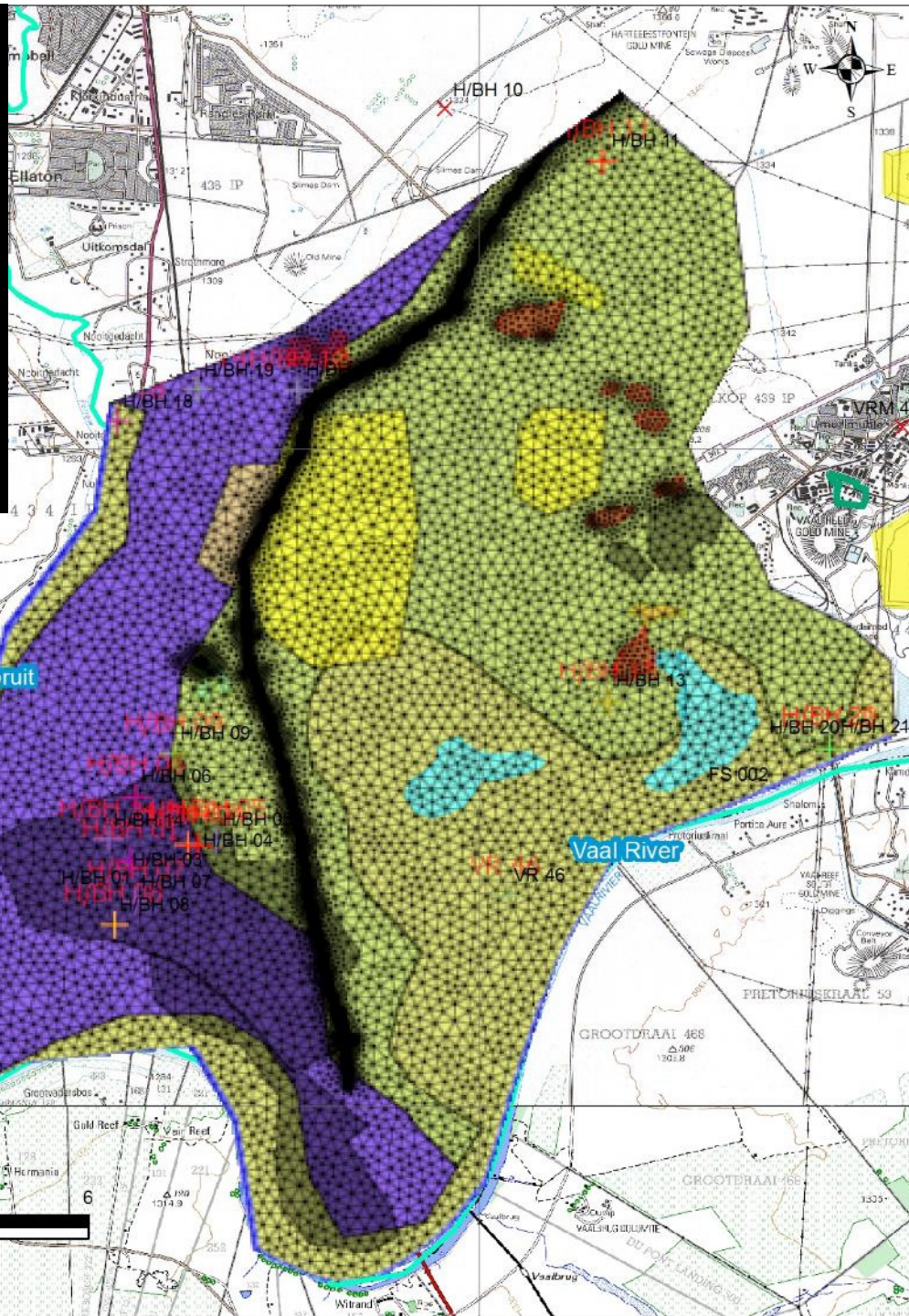
Figure 30: Aquifer delineation and Feflow generated mesh (Triangle method)
