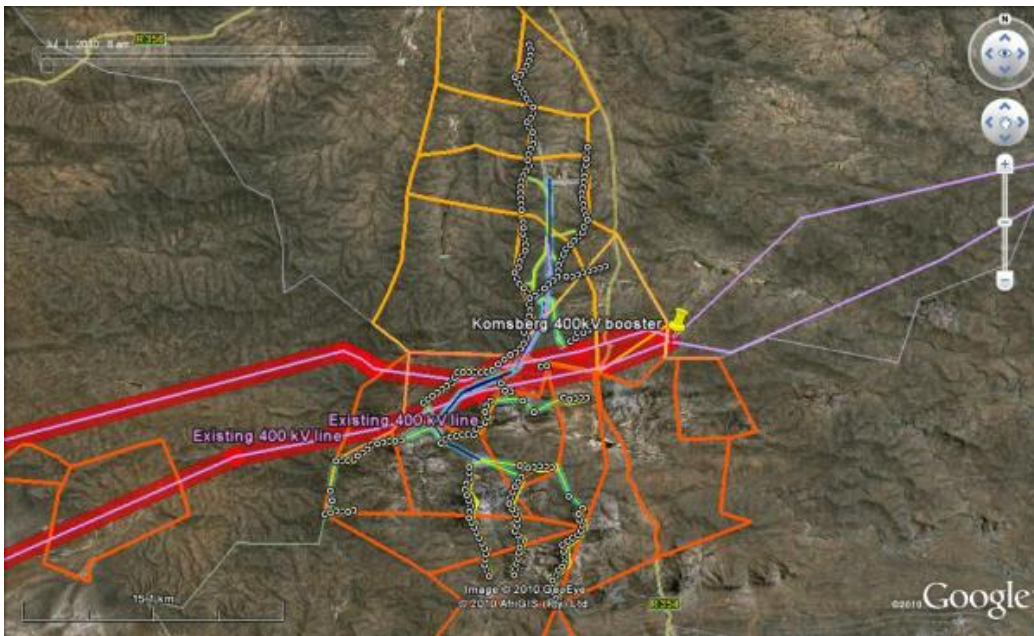
Figure 2.2 Layout and proposed power line link between the Roggeveld WEF and the Komsberg substation.
