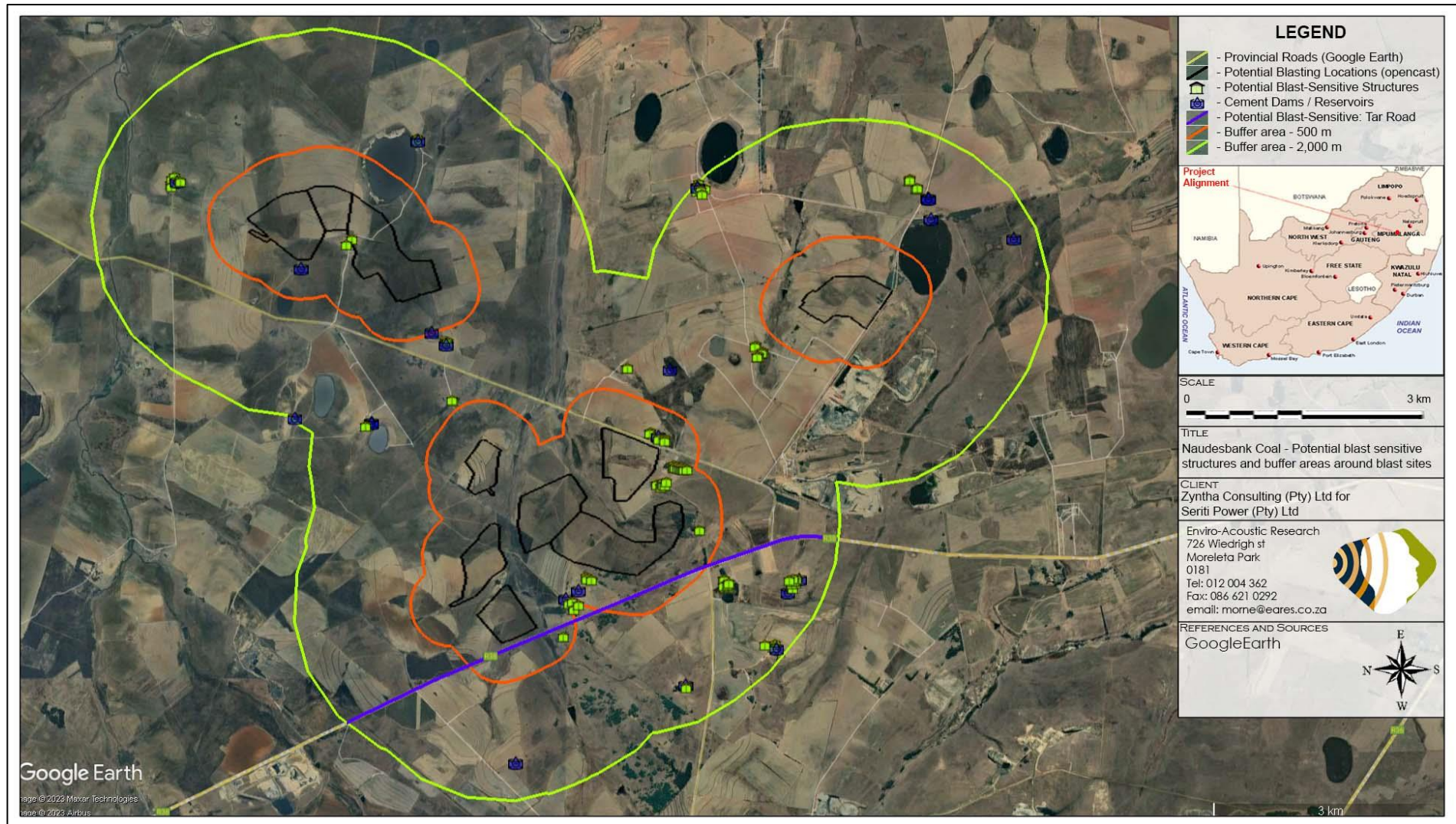
Figure 3-4: Aerial image indicating potential BSS and Infrastructure within 2,000 m of potential blasting areas (opencast areas)
