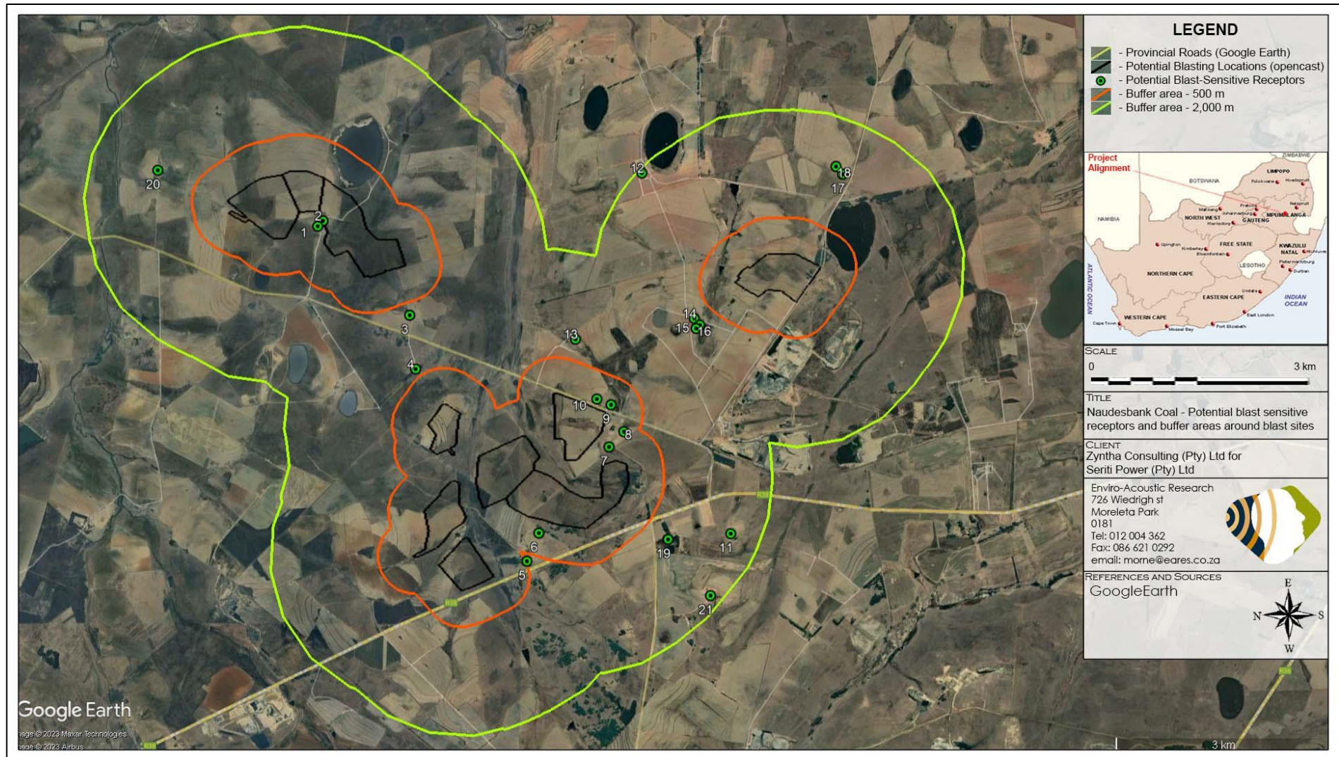
Figure 3-3: Aerial image indicating potential BSR within 2,000 m of potential blasting areas (opencast areas)
