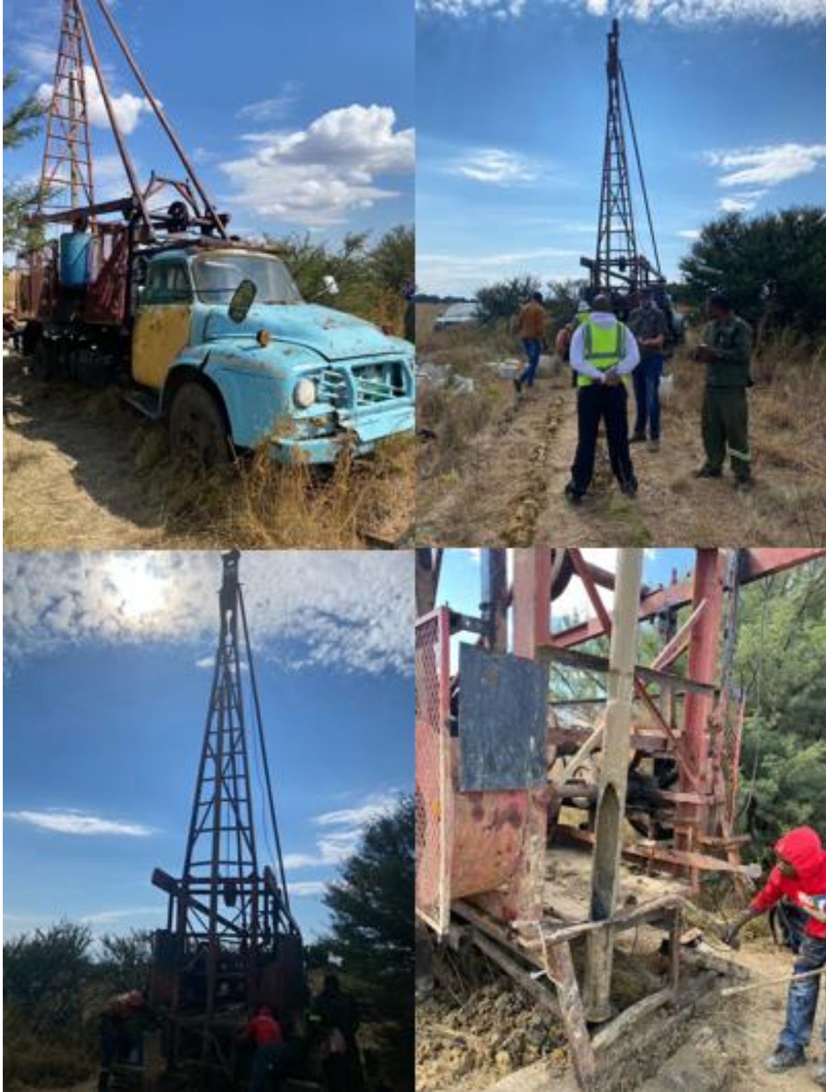
Figure 6-2 Photographs of the jumper rig planned to be used for the programme
