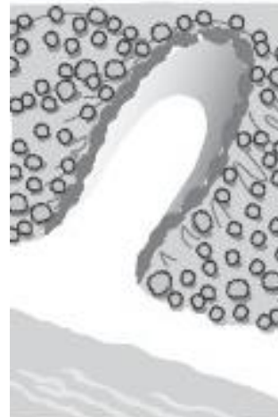
(b) Place brush on exposed areas where blow-out lip has been disturbed.
