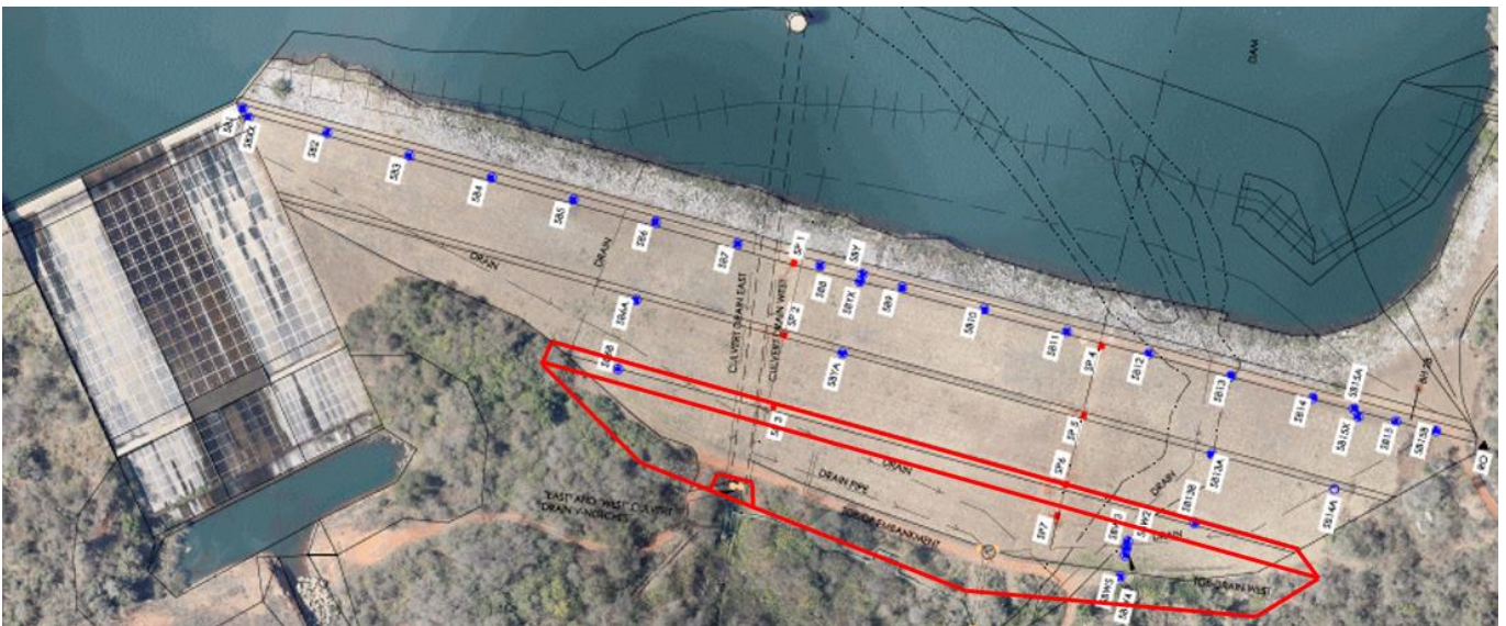
Figure 5: Proposed stabilizing berm on downstream face
