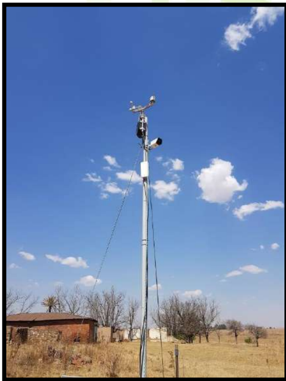
Figure 14: Real Time Indicative Monitor field node
