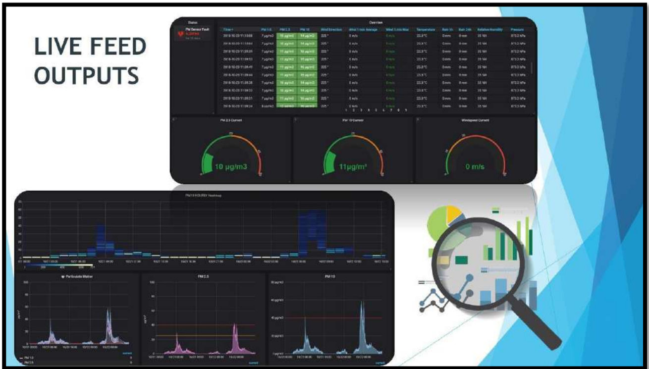
Figure 15: Typical Real-Time Ambient Particulate Matter monitoring dashboard communication interface
