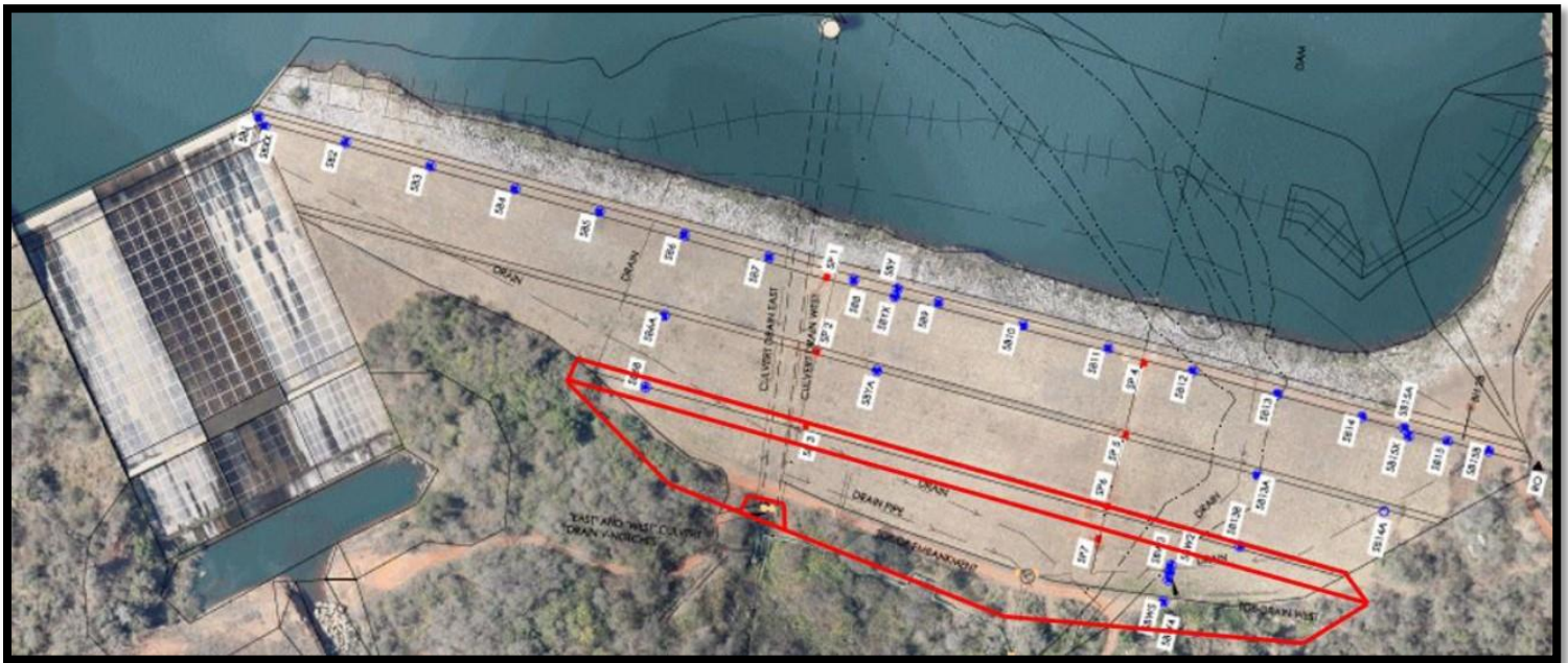
Figure 2: The proposed stabilising berm (red polygon) on downstream face of the Ngodwana Dam wall (Hagen, 2019).
