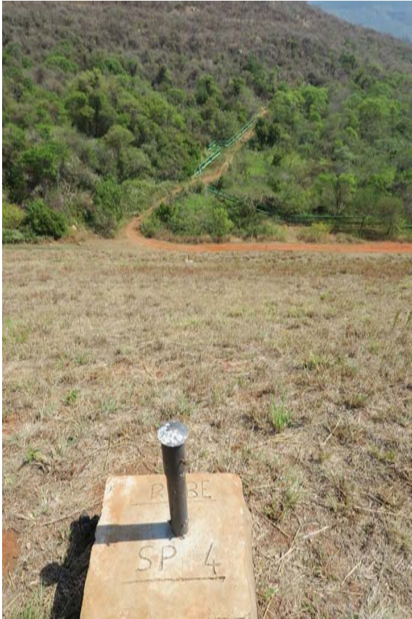
PLATE 3:- Standpipe piezometers SP4-7 along “riverbed” section
