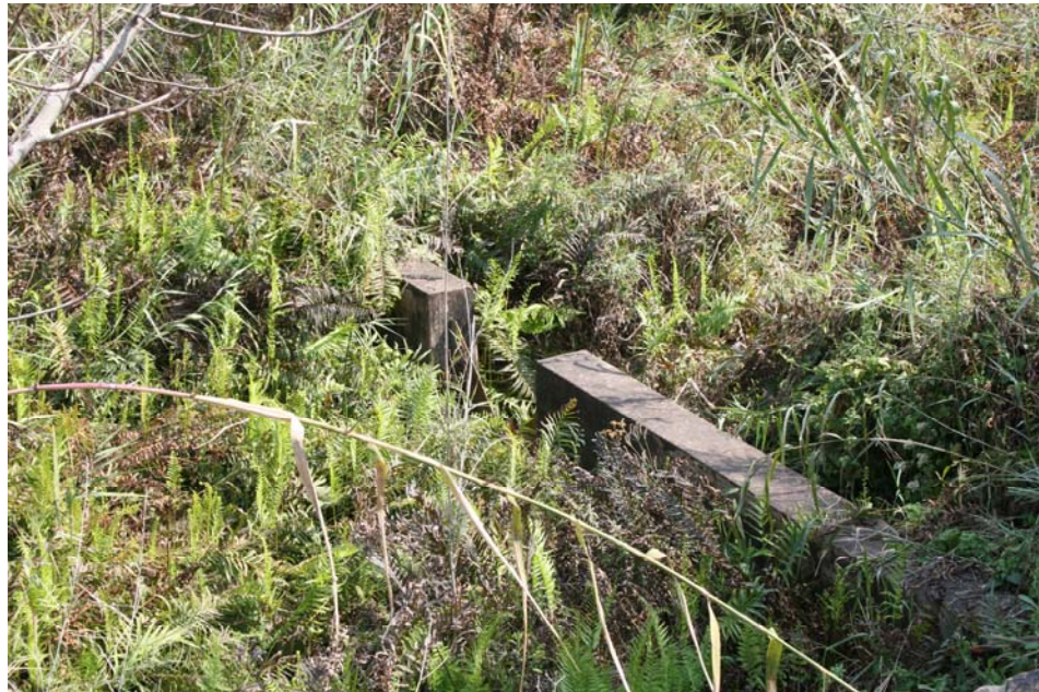
Plate G7. Weir for measuring "Seepage 1".
