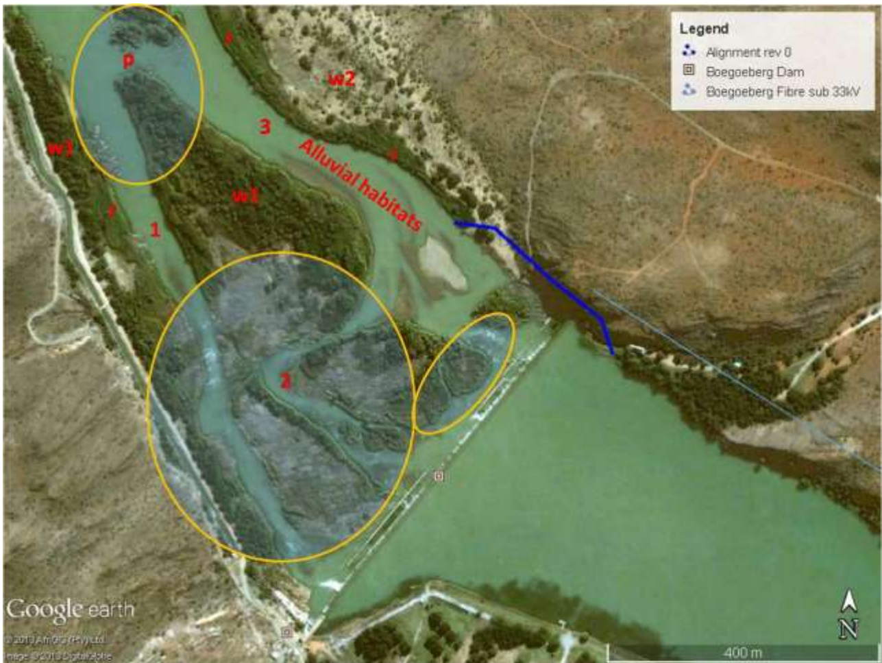
Figure 2.2 Aerial view of the site to be impacted by the proposed development, showing 3 channels that comprise the main Orange River downstream of the dam wall, and the proposed alignment of the hydro scheme (dark blue line).
