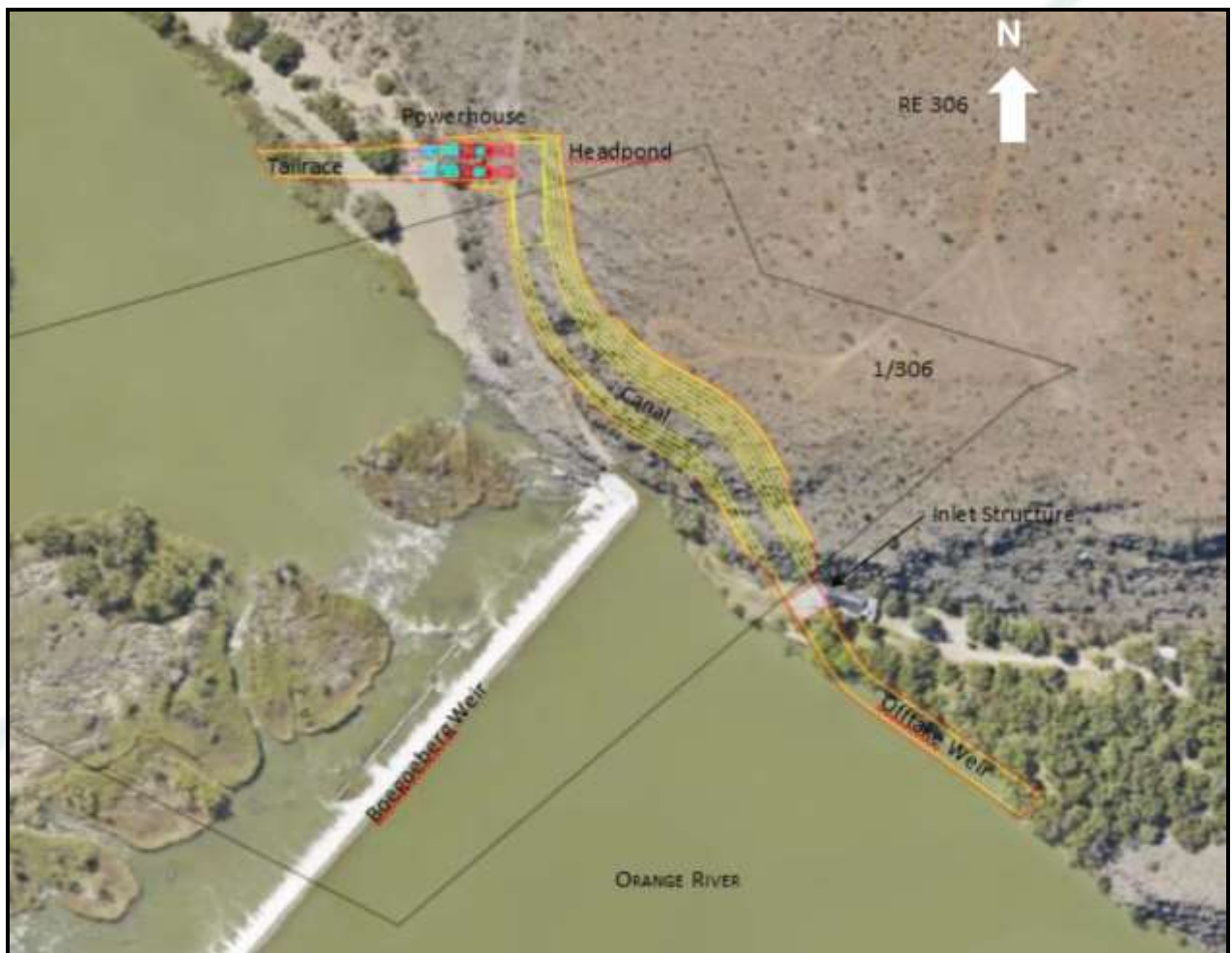
Figure 26. Aerial view of the proposed hydro-power infrastructure at Boegoeberg Dam on the farm Zeekoebaart 306 (Source: Boegoeberg Hydro-Power Final Scoping Report, Aurecon)
