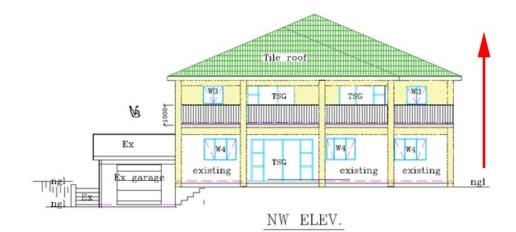
We propose to develop the building towards the back of the site, as this allows us to keep the original aesthetic of the front building face. The back of the site is an open back garden. We will try to reuse as much of the existing roof as possible. Similar windows and doors will be used to promote continuity between existing and new. We will carry up the front columns to support a balcony.
