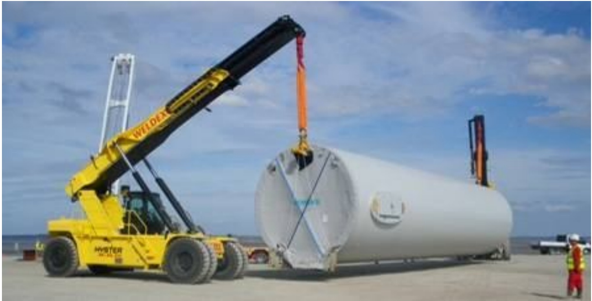
Picture 5: Reach stackers for port // laydown handling.
