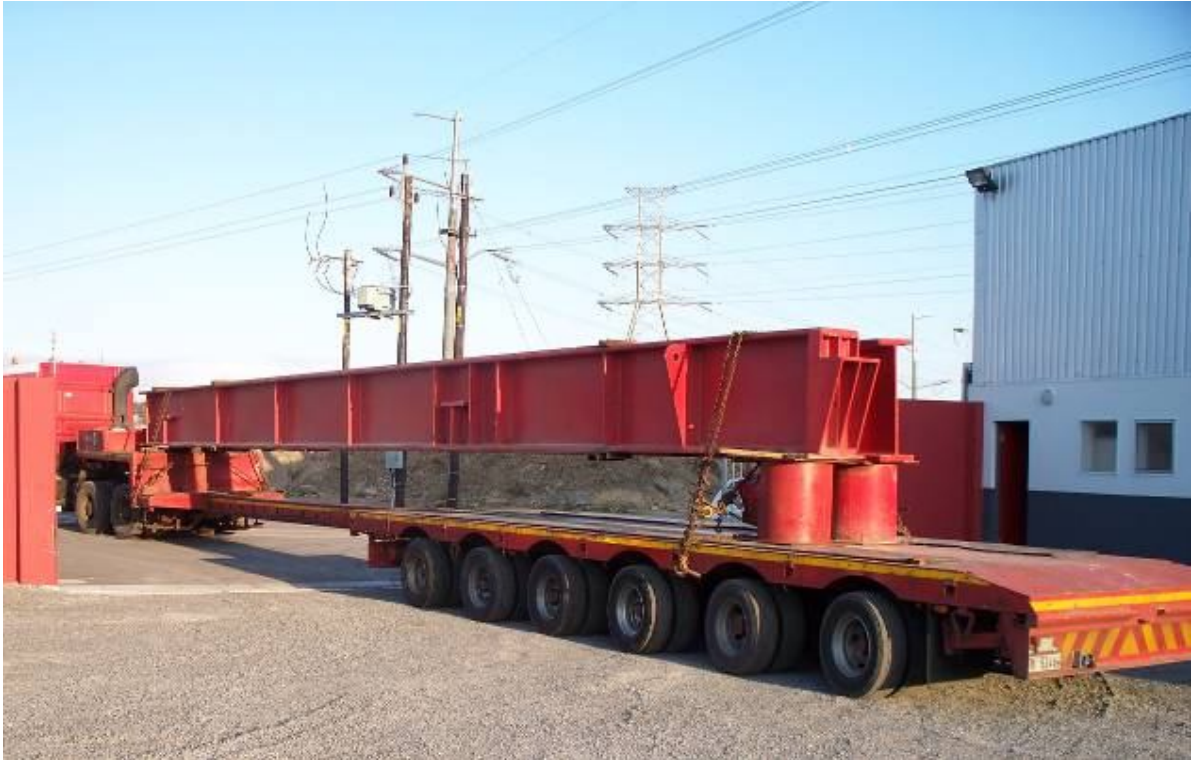
Picture 8: Broshuis 6 axle-line extendable semi-lowloader trailer
