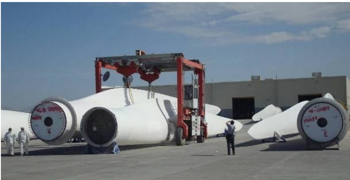
Picture 4: Mobile gantry for port // laydown handling.
