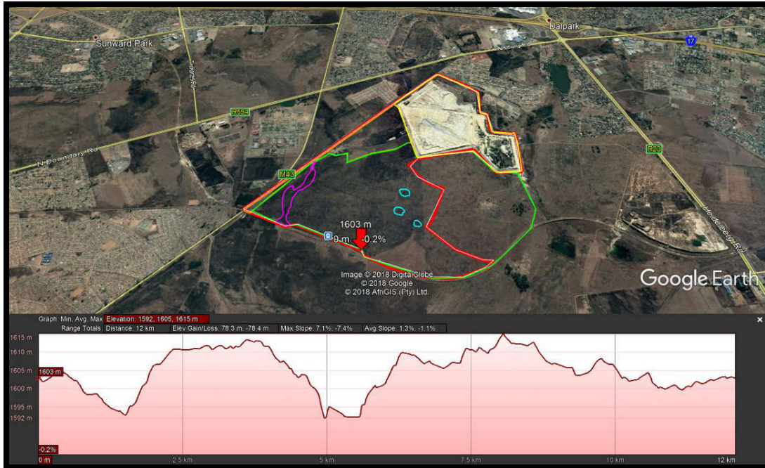
Figure 3. An elevation profile of the site. The site has a gentle sloping topography from the north towards the east with an average slope of 1.3%. The major topographical features are the artificially created mine dumps (old slimes dam) on the northern portion of the site.
