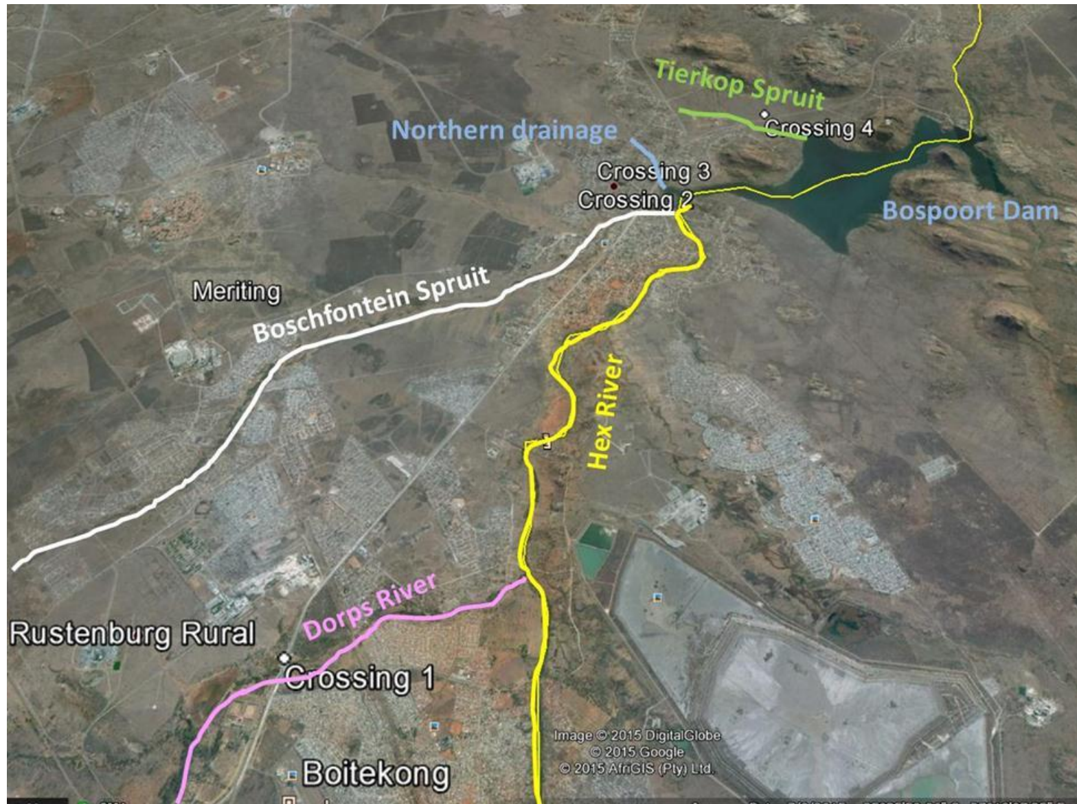
Figure 5: The study area depicting the Hex River and tributaries and the proposed pipeline crossings.
