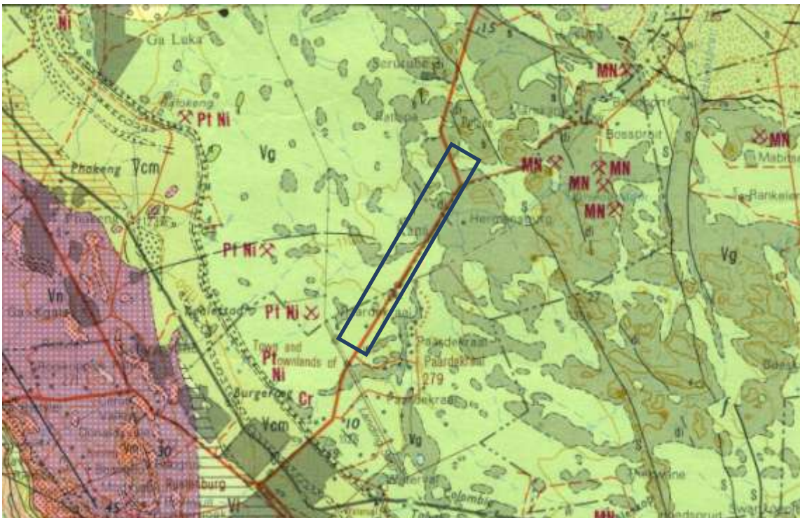
Figure 2: Geological map of the area northeast of Rustenburg and Kana/Kanana. The location of the proposed pipeline routes is within the blue rectangle. Abbreviations of the rock types are explained in Table 2. Map enlarged from the Geological Survey map 1: 250 000 2526 Rustenburg, 1981.
