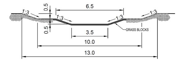
The maximum flow depth during a 1:100 year flood will approximately be 0.84m. The channel will mainly consist of grass and grass blocks to ensure a natural feel to the channel. Grass blocks will only be installed in the low flow channel to ensure soil protection during high flow rates.
