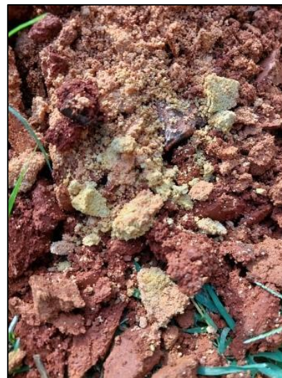
Plates 29 & 30: Spoils retrieved from AH1 (left) and AH2 (right) showing a thin layer of colluvium (dark brown sandy clays) overlying residual dolerite soils (reddish clays) which further overly residual sandstone soils (light brown sands)
