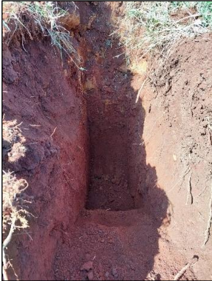
Plates 22 & 23: Colluvium overlying residual dolerite soils comprising sandy clays with occasional dolerite and sandstone boulders
