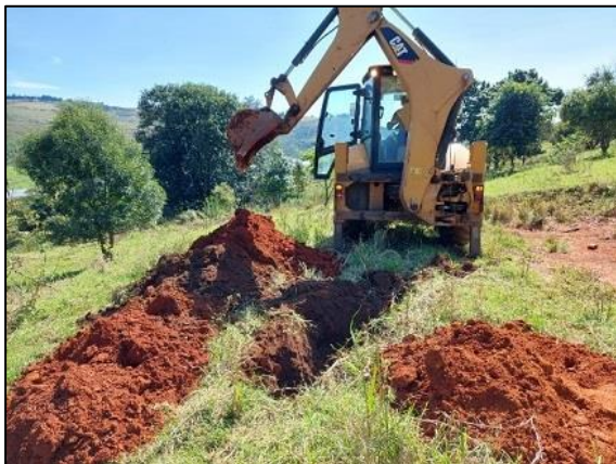
Plates 24 & 25: Residual Dolerite soils overlying residual sandstone comprising clayey sands
