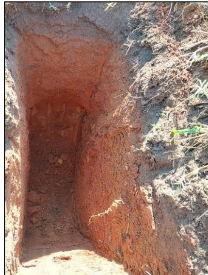
Plates 24 & 25: Residual Dolerite soils overlying residual sandstone comprising clayey sands
