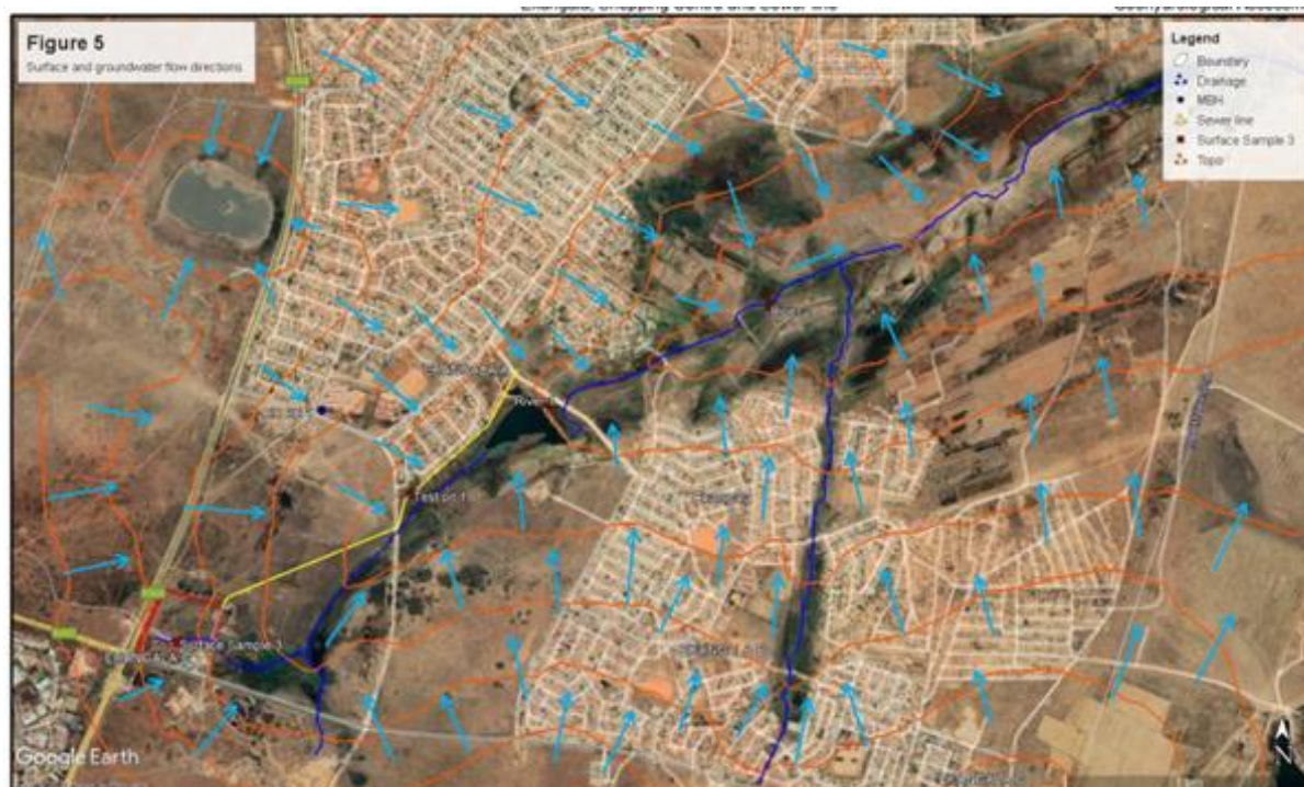
Figure 3: Groundwater flow direction
