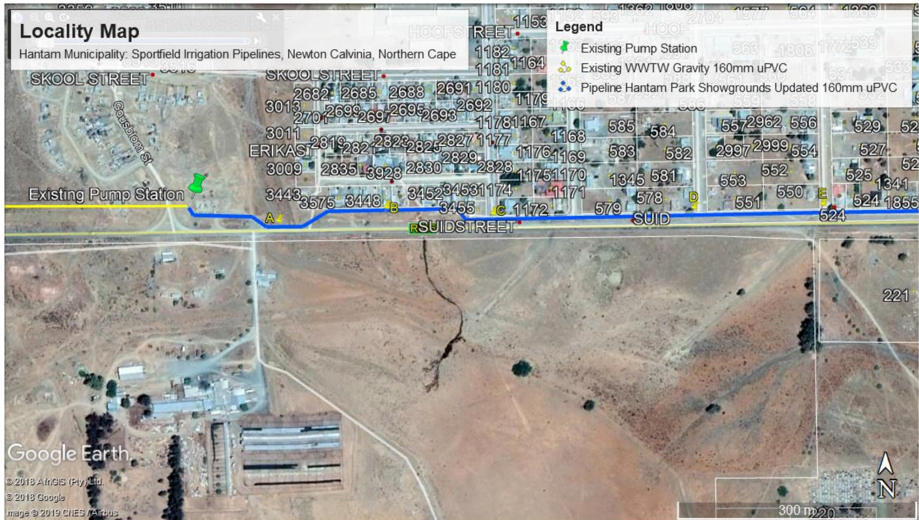
Figure 5: Google map focussing on the pipeline to Hantam Park Showgrounds (blue) from the existing pump station until point E. Pipeline to cross a culvert at point A over an existing structure. Pipeline to remain on gravel roads and municipal land.
