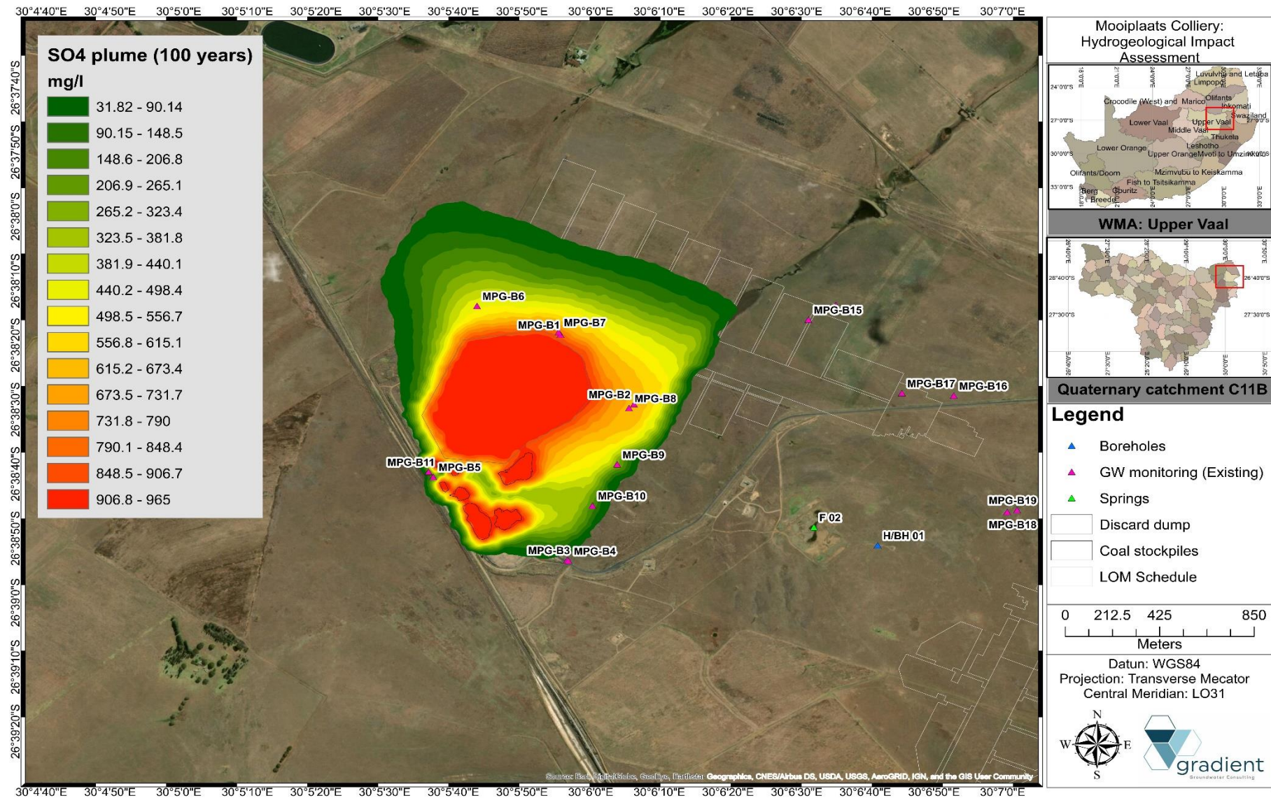
Figure 12-28 Scenario 03c: Post-closure sulphate pollution plume (100 years)
