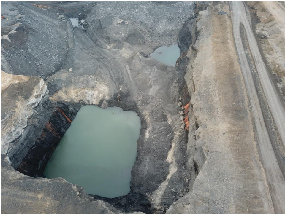
FIGURE 53: ORANGE SEEPAGE INDICATIVE OF AMD LEACHING INTO THE PIT
