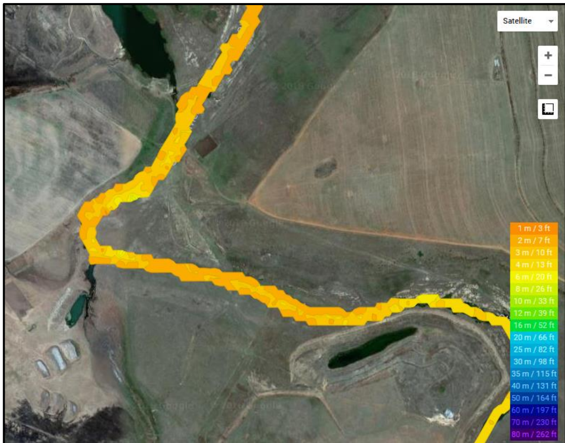
FIGURE 27: BATHOMETRIC RESULTS FOR THE DIVERSION AREA
