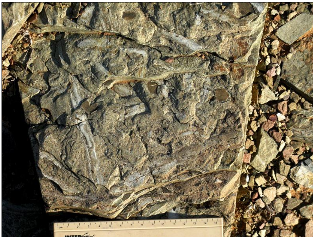
Figure 12. Well-consolidated, laminated, fine-grained sandstones of the Prince Albert Formation exposed in hillslopes just NW of the borrow pit study area showing pale strap-shaped burrows at several successive horizons (Scale in cm).
