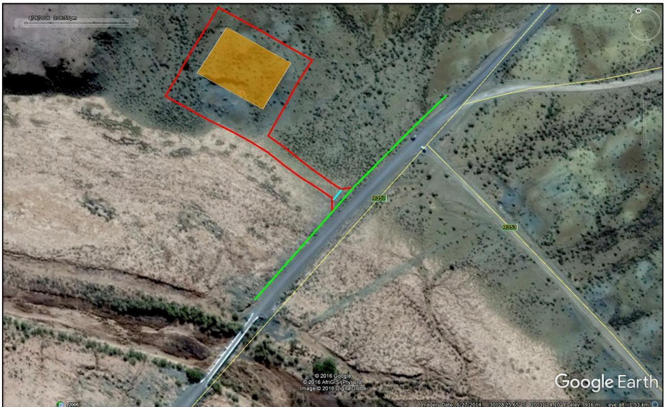
Figure 3. Google satellite map of the borrow pit study area (red polygon) on the eastern side of the Sak River, showing the location of the existing pit as well as the proposed new excavation area (orange rectangle), as well as the access road to the tar road (EnviroAfrica 2017).
