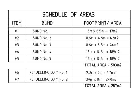
TOTAL PROPOSED SITE CAPACITY =  $5 \times 83m3 + 1 \times 23 m3 + 1 \times 14m3$ = 452m3 THIS DRAWING MAY NOT BE LENT, COPIED OR REPRODUCED IN ANY WAY WITHOUT THE PERMISSION OF PETROLEUM SOLUTIONS.
