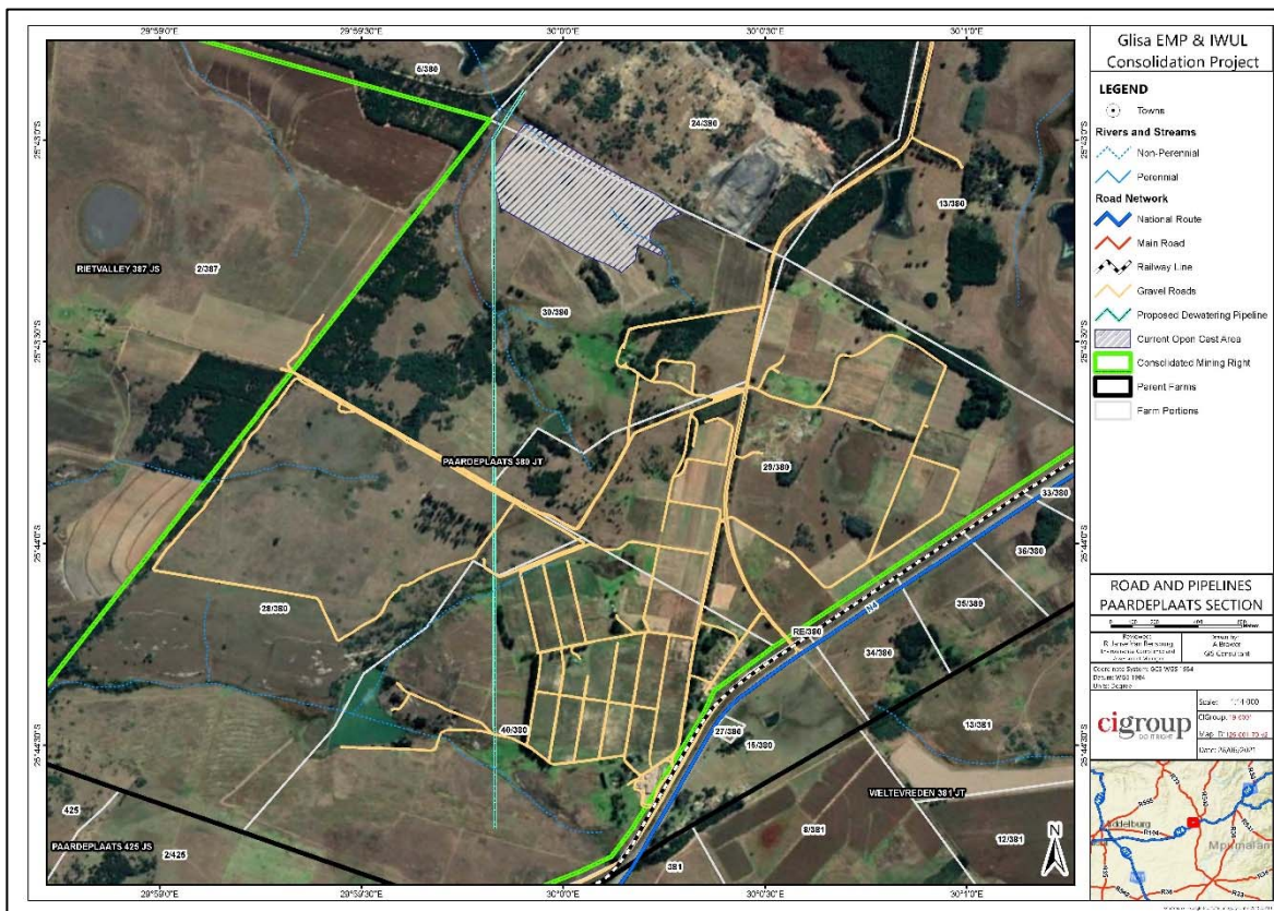
Figure 2.8: Proposed Gravel Haul Roads and Dewatering Pipeline in the Active and Planned Mining Areas.
