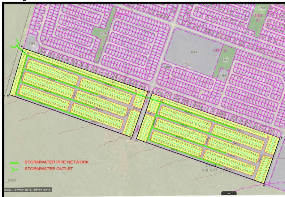
Internal Stormwater layout
