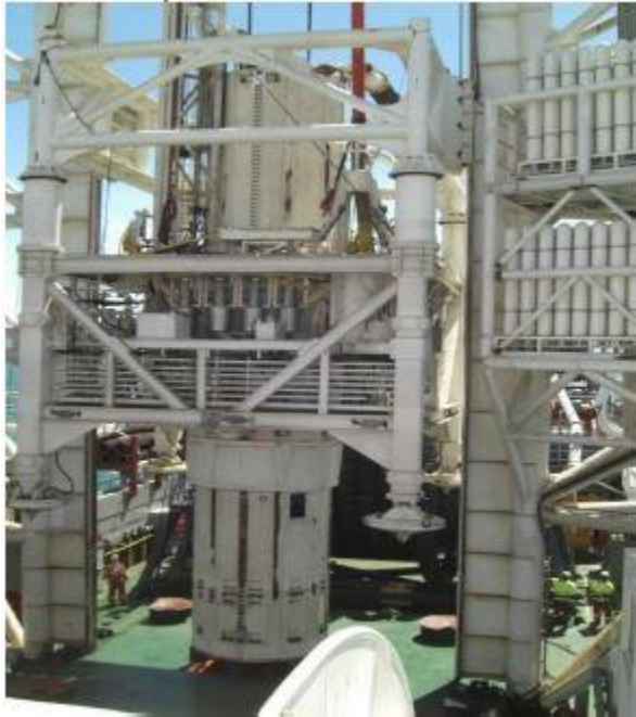
Figure 3: Illustrative example of a drill bit operated from a drill frame structure located onboard a vessel of opportunity.
