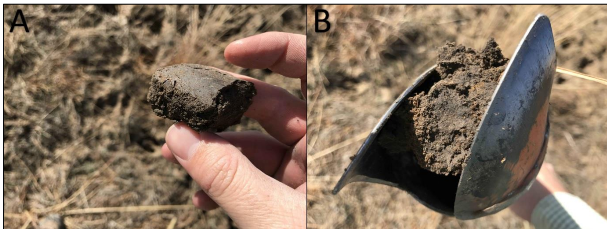
Figure 7-9 Soil horizons identified on-site. A) Ped with slick-and-slide properties. B) Vertic topsoil.
