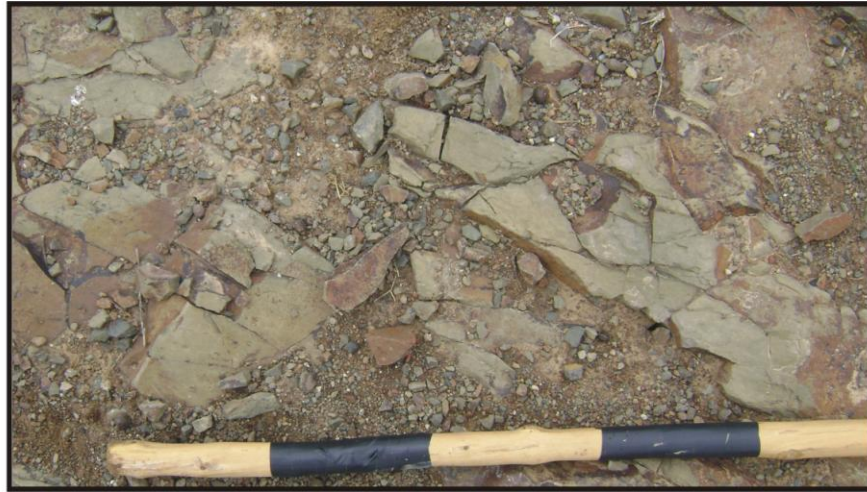
Figure 6. The site is underlain by sedimentary rocks of the Middleton Formation of the (Adelaide Subgroup, Beaufort Group), which is made up of upward-fining, lenticular sandstone grading into mudstone, with prominent red-coloured mudstone beds
