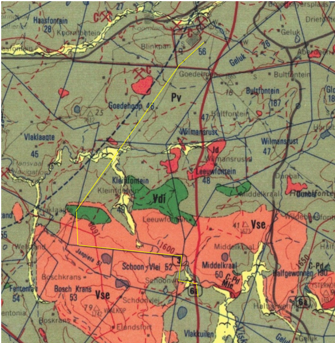
Figure 3: Geological map of the area around the proposed Kudu-Elders powerline route. Abbreviations of the rock types are explained in Table 2. Map enlarged from the Geological Survey 1: 250 000 map 2628 East Rand.
