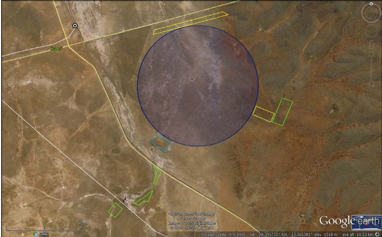
Figure 1. Layout of the ACWA Power SolarReserve Redstone Solar Thermal Power Plant with associated infrastructure. The Project is illustrated in blue with the evaporation ponds in blue while laydown areas are in yellow and management camps in yellow. It is important to note that the satellite image is several years old and does not show the two completed 75MW PV facilities which are also present at the site and which take up a large area to the east and south-east of the Project area.
