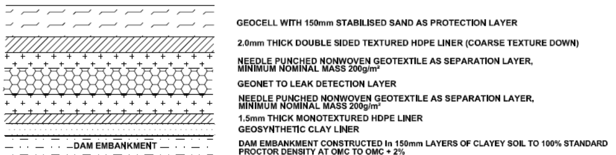
Figure 5. Pollution Control Dam Side Slope Liner Detail
