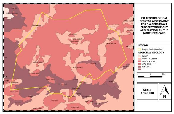
Figure 6: Approximate location and surface geology of the proposed Jaagers Plaat prospecting area in the Northern Cape<sup>1</sup>. Map drawn by QGIS Desktop 2.18.28
