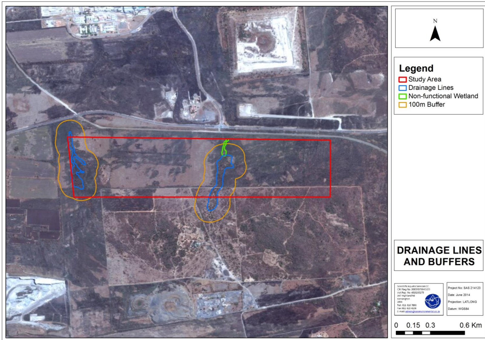
Figure 20: Conceptual representation of the drainage line features present within the study area with associated buffers.
