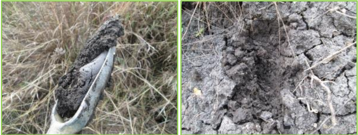
Figure 19: Representative photographs of the soil profile in Drainage Line A (left) and Drainage Line B (right) showing the presence of gleying.
