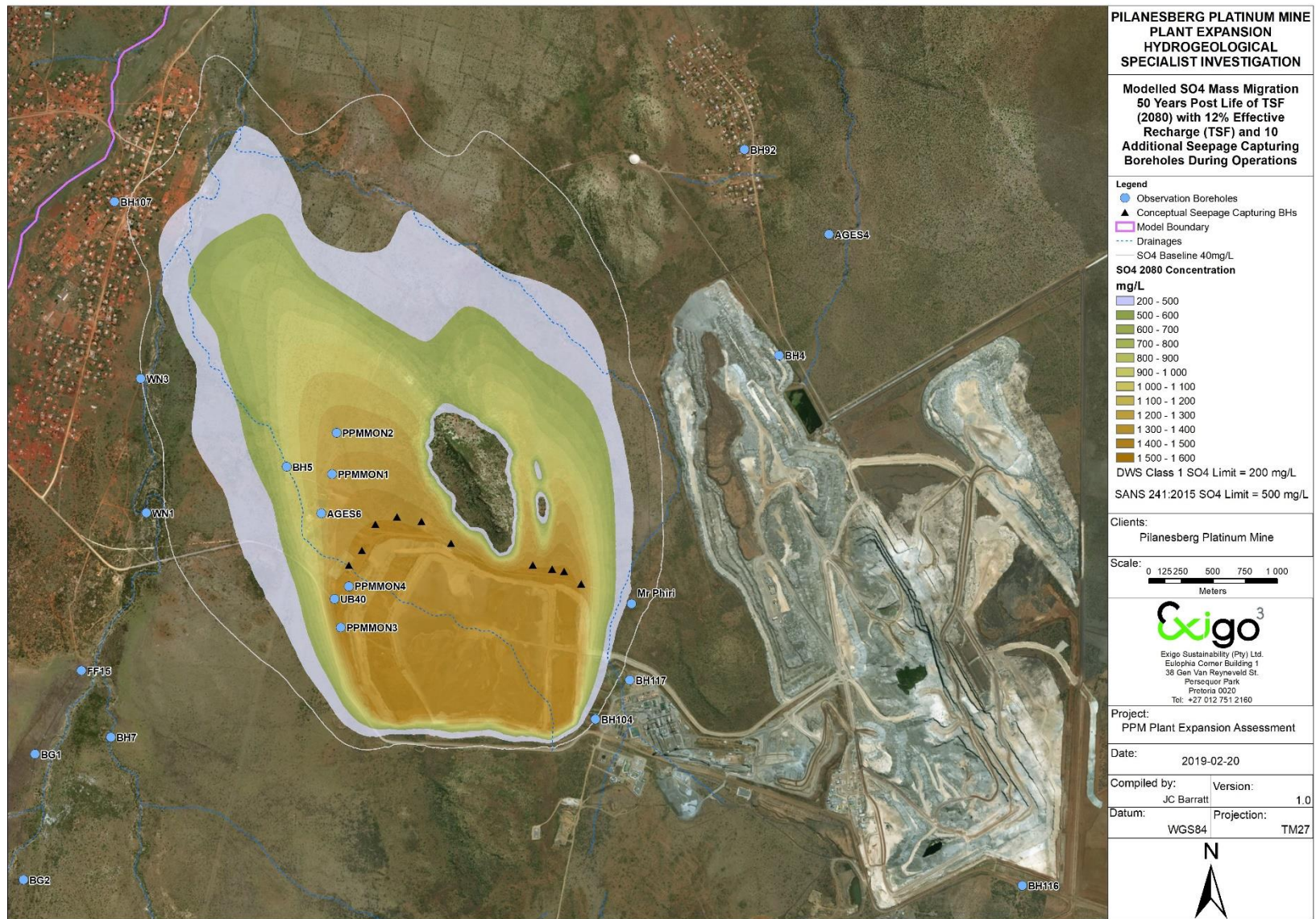
Figure 6-6 Scenario 3b: Sulphate migration with 12% effective recharge by the end of 2080 with 10 additional seepage capturing boreholes
