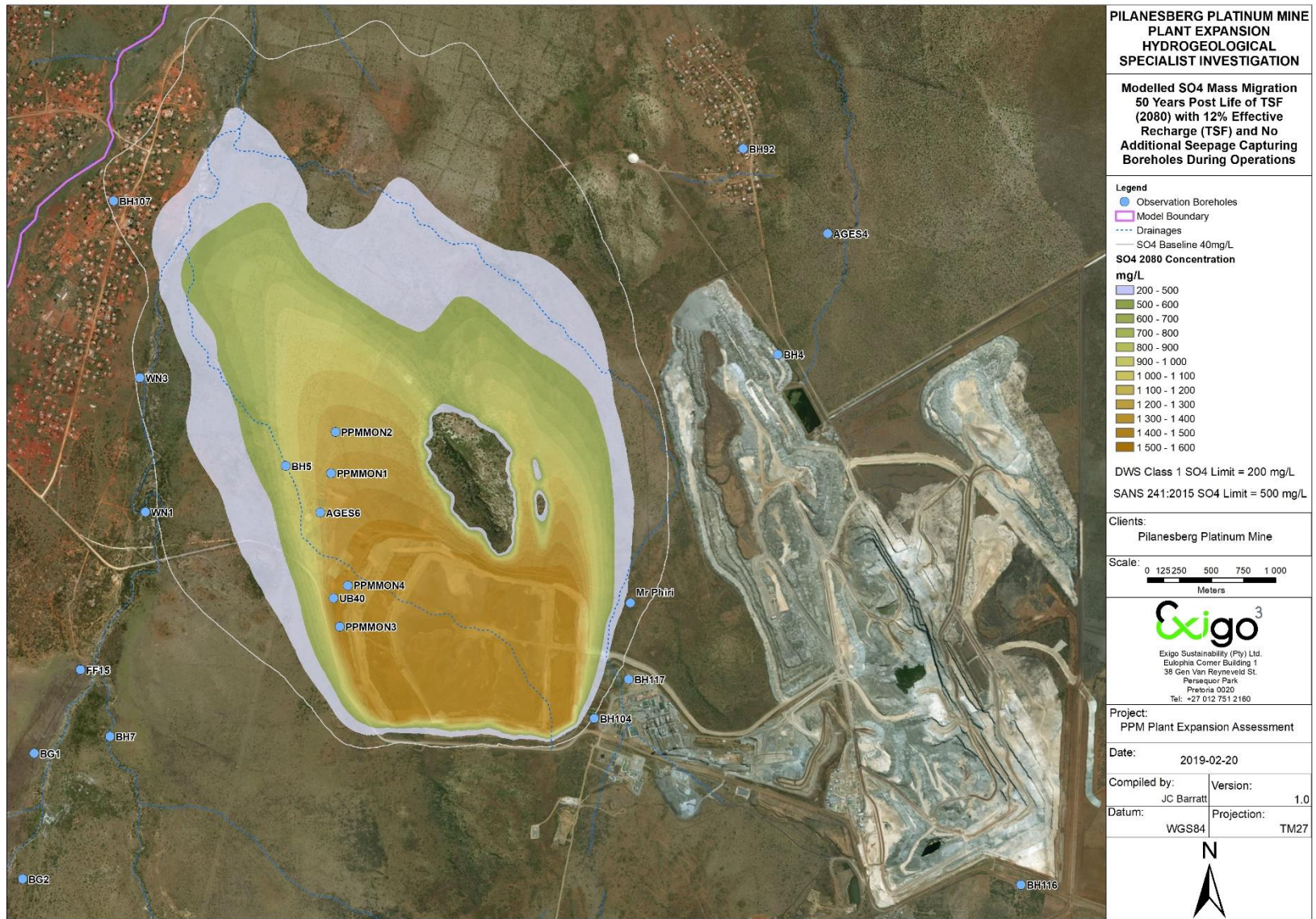
Figure 6-5 Scenario 3a: Sulphate migration with 12% effective recharge by the end of 2080 without any additional seepage capturing boreholes
