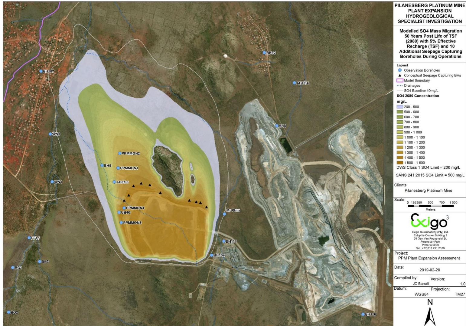
Figure 6-8 Scenario 3d: Sulphate migration with 5% effective recharge by the end of 2080 with 10 additional seepage capturing boreholes
