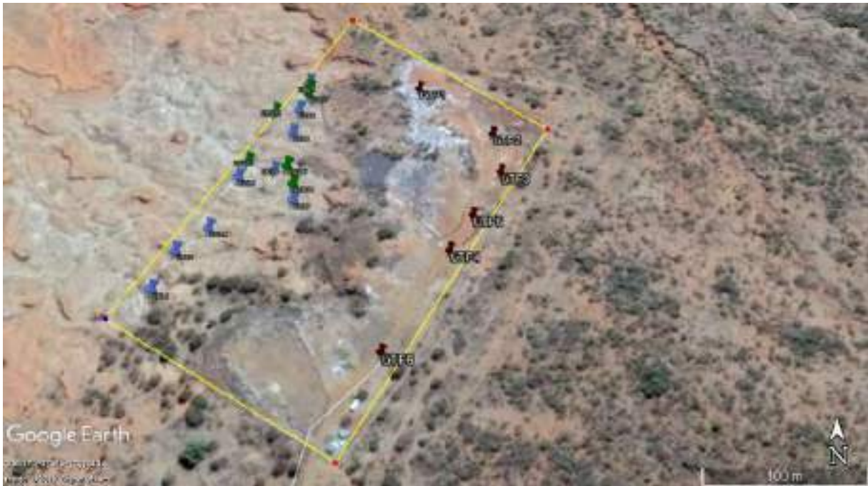
Figure 16: Location of test pits (brown), sandstone (green) rock in-situ exposure and positions of dolerite (blue) boulders mapped against the landfill boundary fence (yellow).
