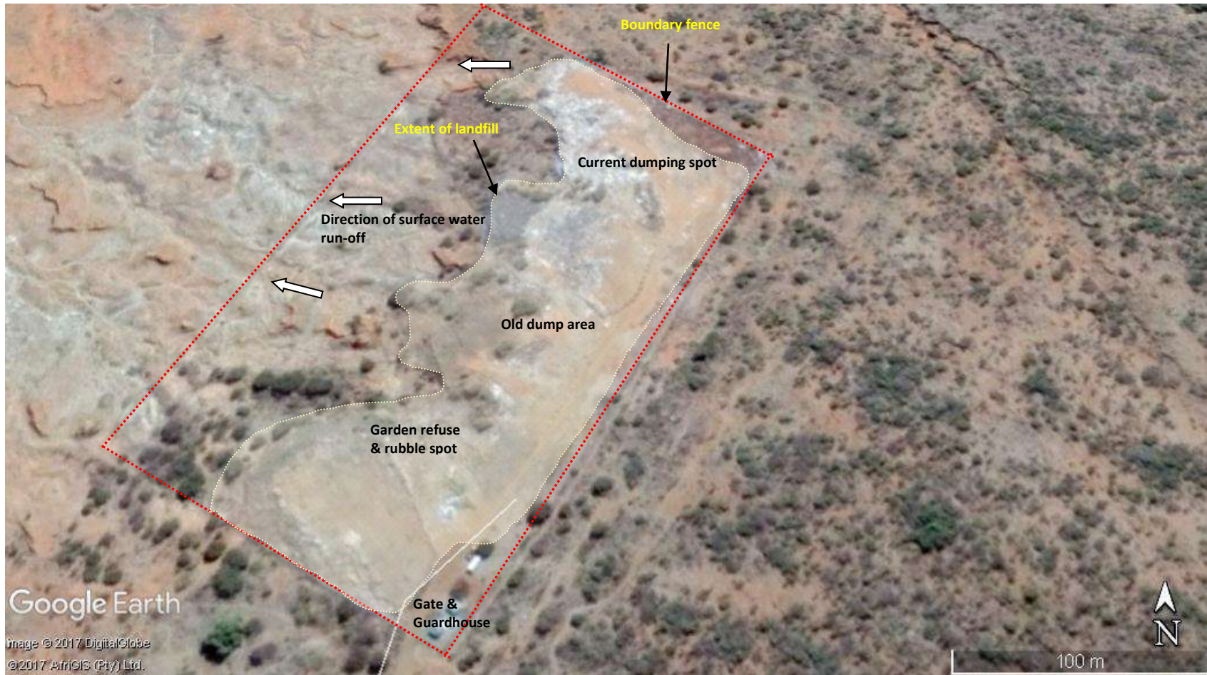
Figure 13: Planview showing fenced area of the landfill, extent of landfill deposition to date and direction of drainage water flow.
