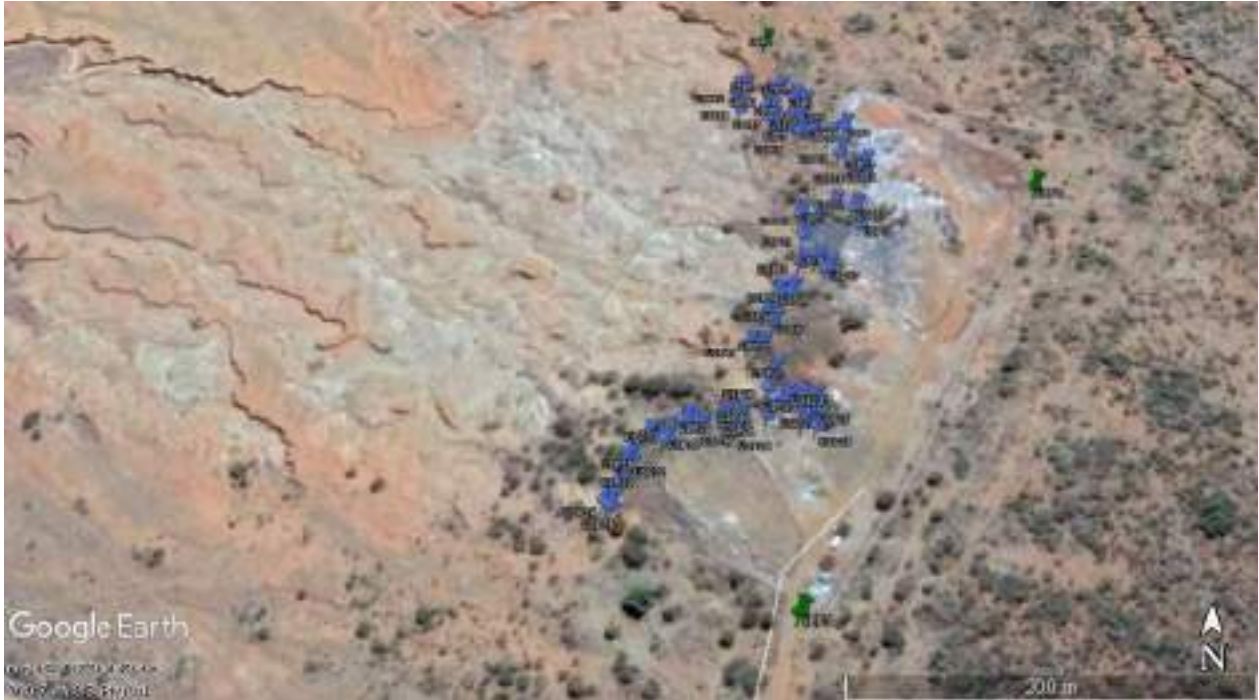
Figure 15: Example of locations of survey points (fence boundary corners – green) and landfill surface extent and slope elevations (blue).
