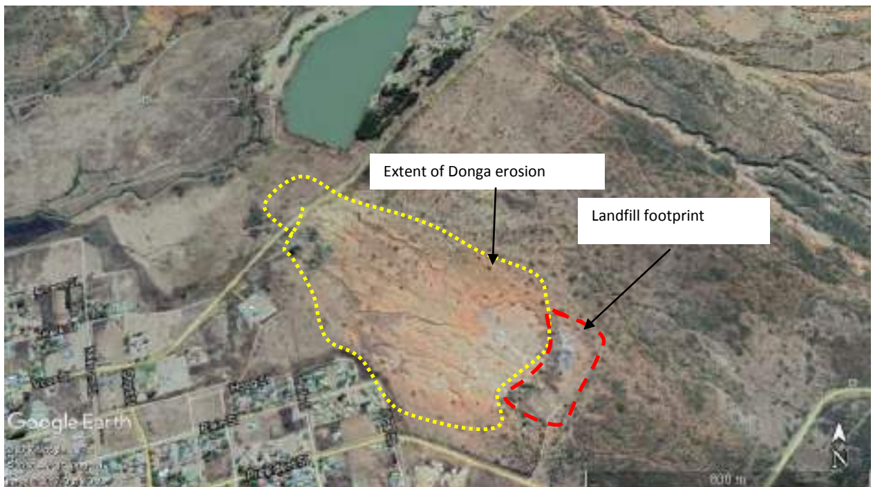
Figure 2: Extent of donga erosion with direction of water and sediment flow in the NW direction. Location of surface water bodies in the area (river and dam).
