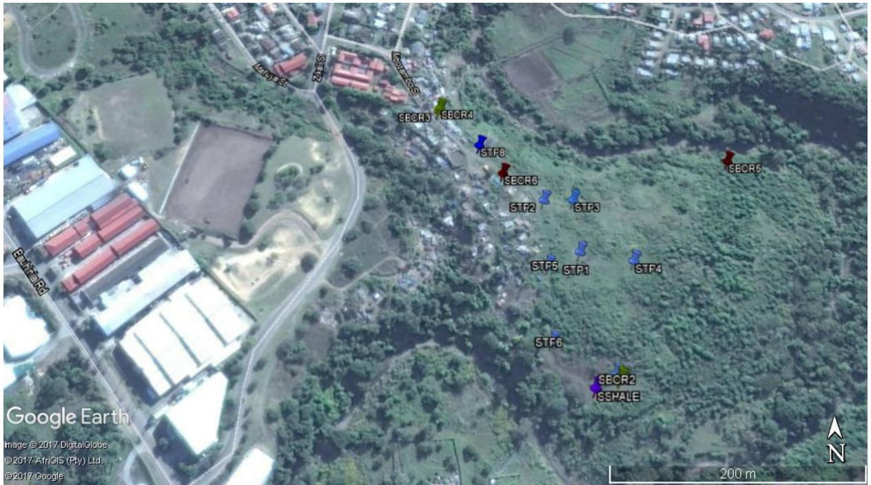
Figure 10: Location of 8 test pits (blue), Monitoring boreholes (green), unknown boreholes (brown) and shale geological exposures (navy).
