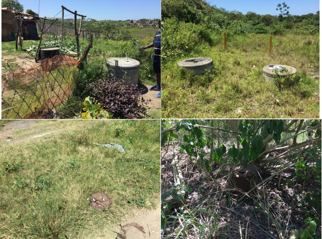
Figure 20: Sealed x2 monitoring boreholes (top) and x2 drilled boreholes (bottom).
