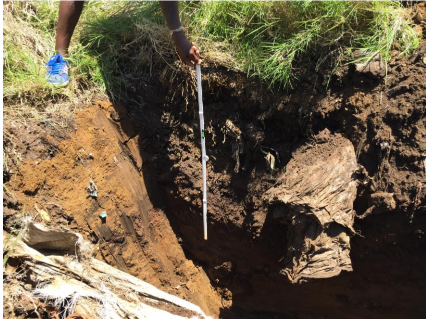
Figure 15: STP5 test pit profile showing capping soil over waste.
