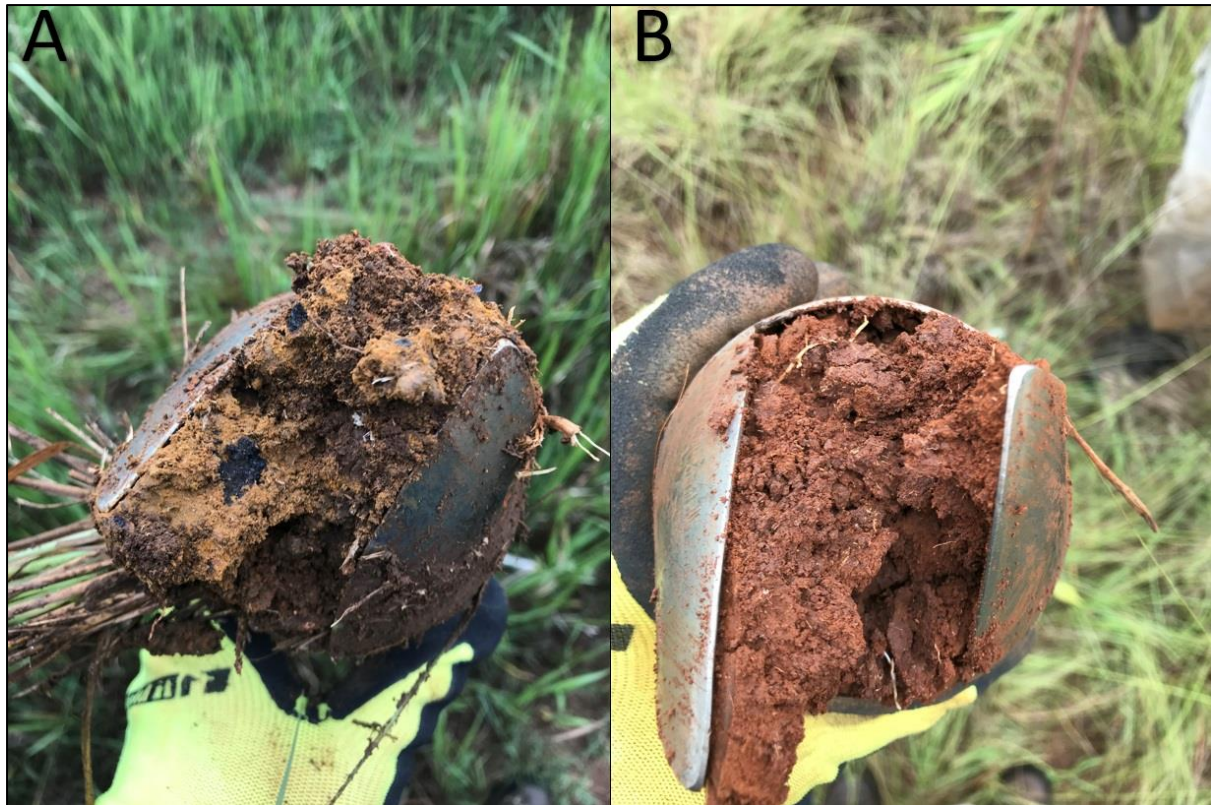
Figure 7-6 Relevant soil horizons. A-Soft Plinthic horizon. B-Red Structured horizon
