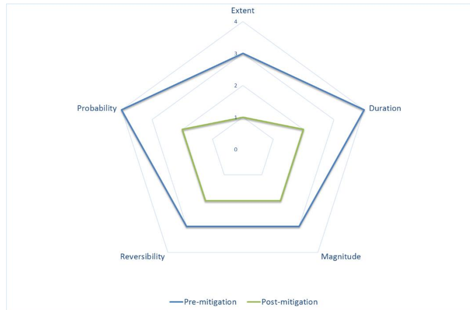
Figure 7-10: Radar plot indicating the pre – and post mitigation impacts associated with erosion and sedimentation during operation – Alternative 1.
