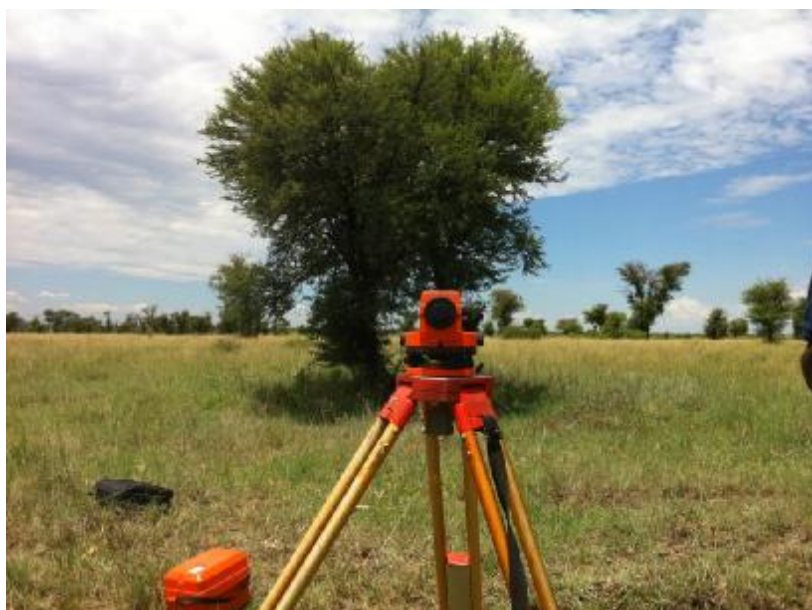
Figure C5: View of dumpy level and reference point (tree) on the right bank at cross-section in Bofule River
