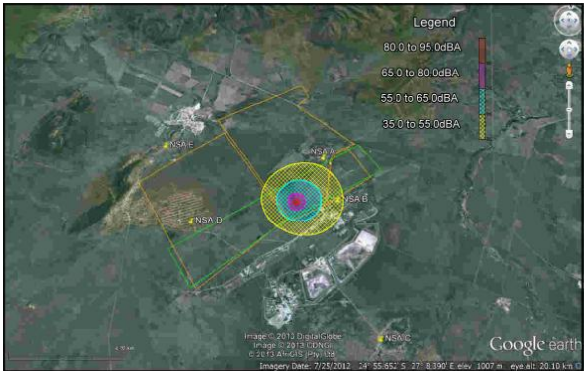
Figure 6: Noise contours for the open cast pit activities
