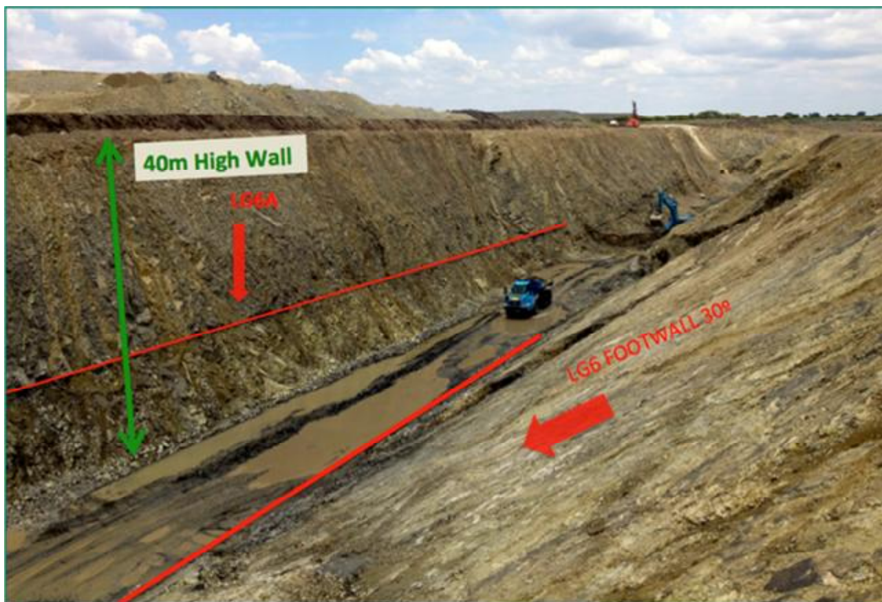
Figure 17: Opencast layout of the LG6 and LG6A chromitite seams at BCR mine
