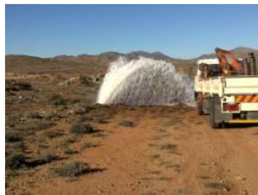
Typical pressure bursts occurring due to deterioration of the pipe wall thickness
