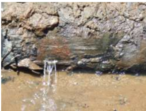
Typical pressure bursts occurring due to deterioration of the pipe wall thickness
