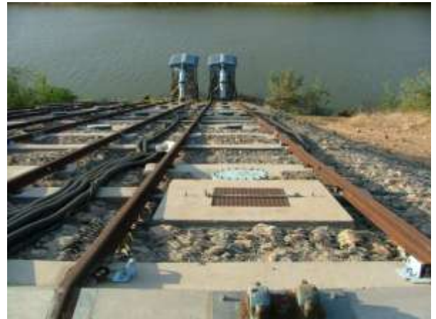
Typical examples of pumps on a trolley configuration
