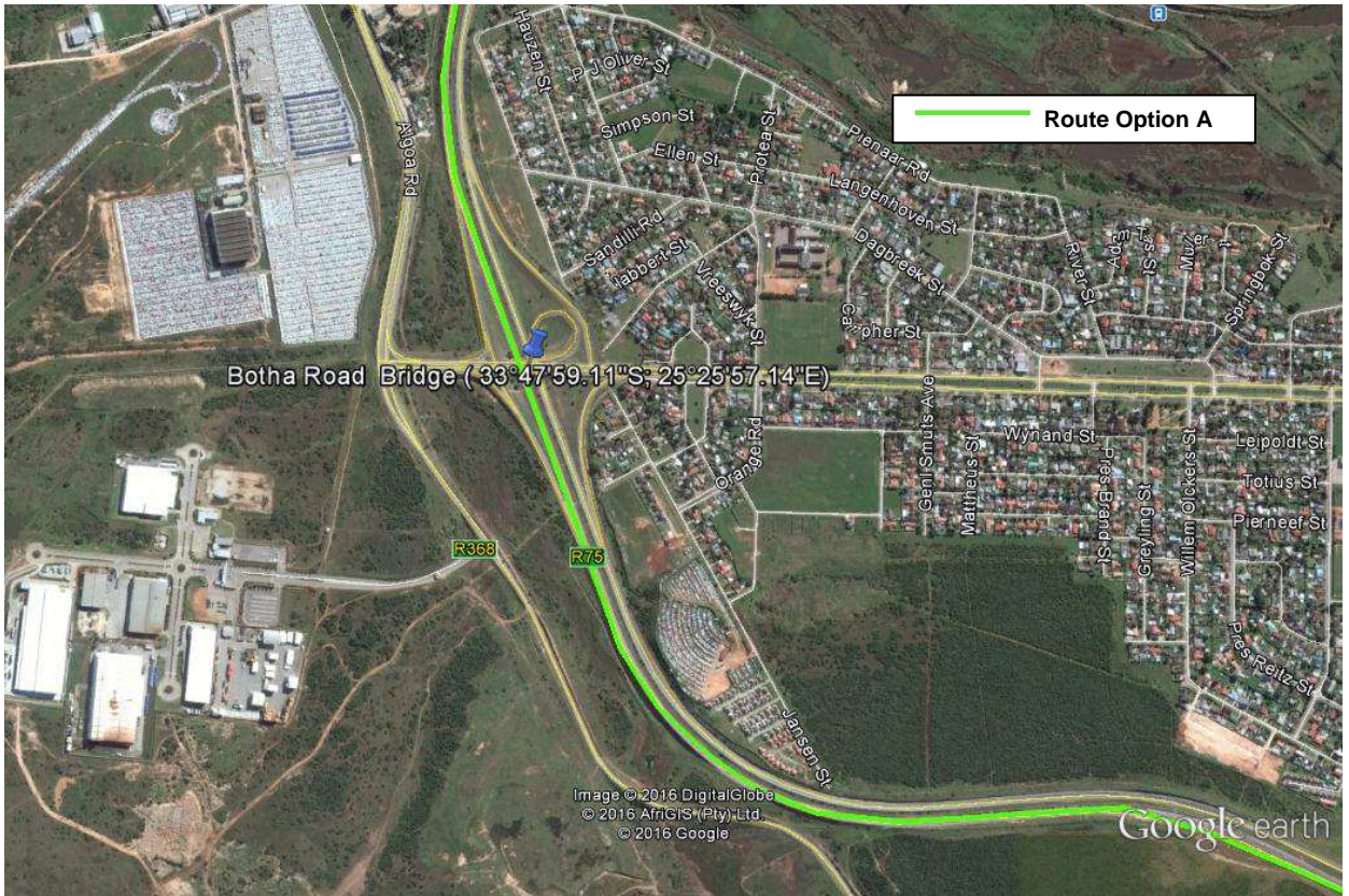
Google Image 15: Continue northwards on the R75 crossing the Botha Road Bridge. The bridge has a clearance of more than 5.5m. (See image below).
