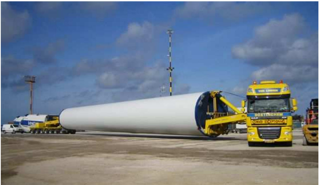
Photo 3 : Tower Sections transported with trucks equipped with the Schnable Connection to reduce the total load height. Height clearances required can be as low as 4,8m at the extreme.
