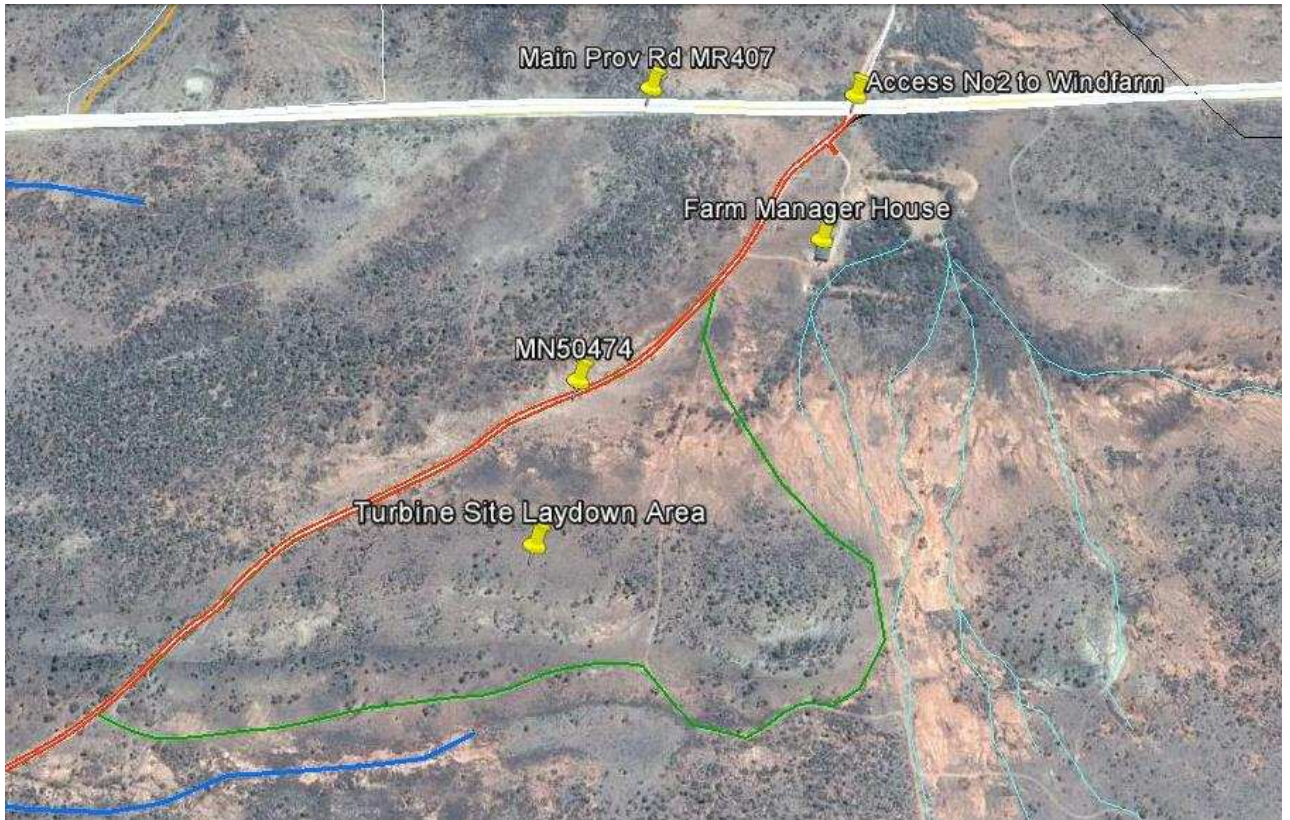
Google Image 31: Access Roads and locality of the proposed centralised “ Turbine Component Laydown Area ” at position : 33°31'54.76"S and 25°03'51.06"E. It is recommended that all turbine components be transported directly / as soon as possible, from the Ngqura Harbour, to this area for the temporary holding of WTG components. Mobile cranes will be required at this area for the safe handling, off-loading and loading.
