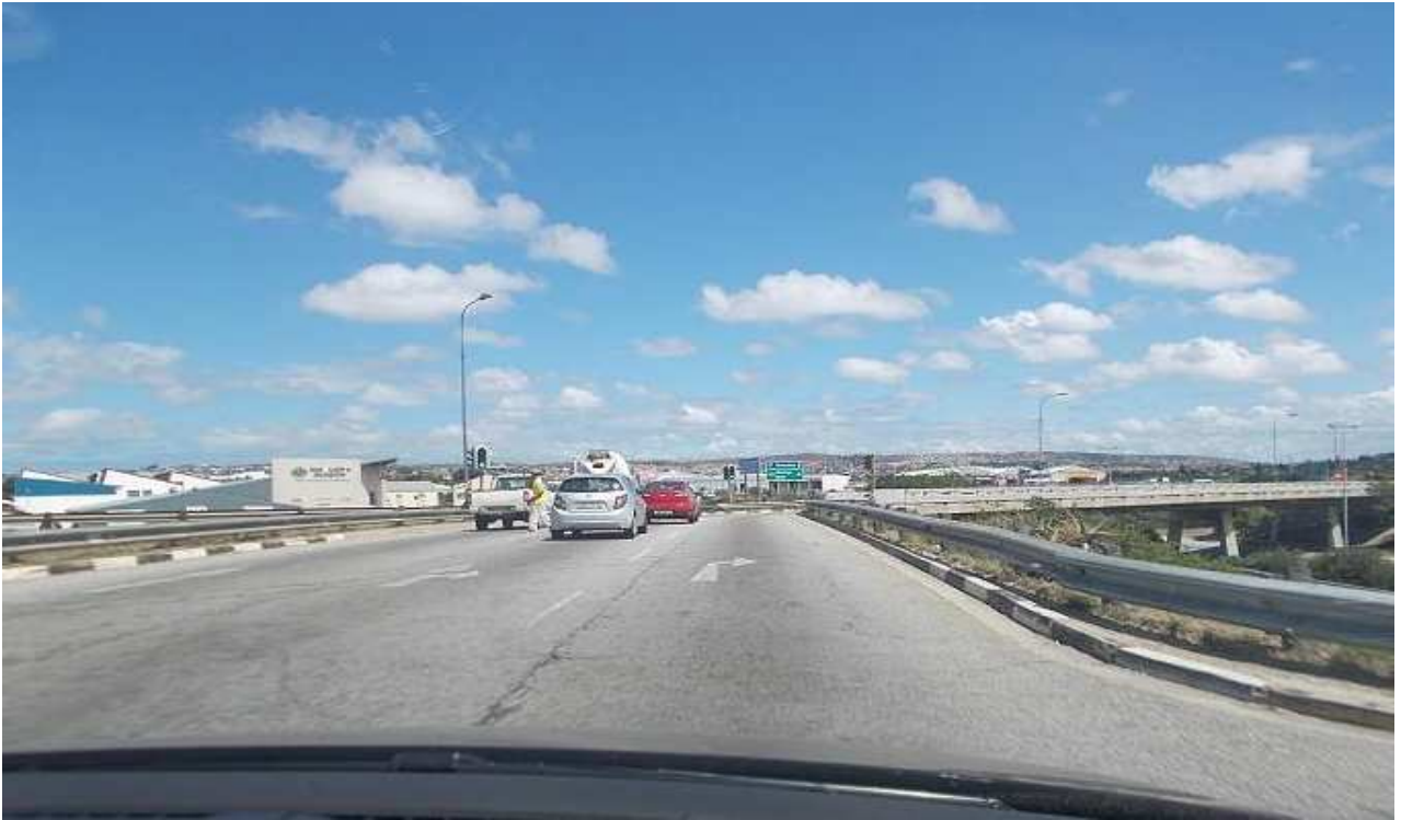
Photo 2: View of the N2 with the off-ramp to the R75. Sufficient space for right turning manoeuvres by transport vehicles, especially for turbine blades may not be available. It is not possible to widen the intersection to accommodate turbine component transportation. This is also a very busy intersection with heavily congested traffic. Traffic police escorts will be required to assist and control the traffic, which may include temporary traffic stoppages while turning right onto the R75 ramp.
