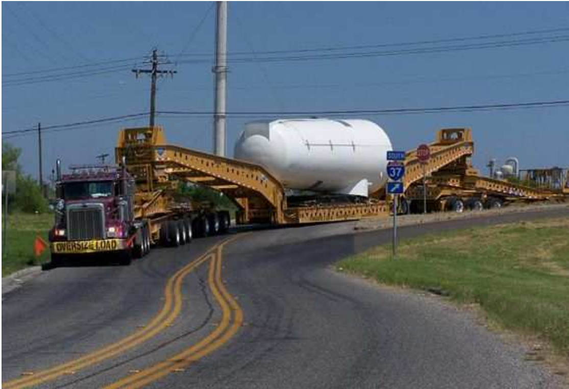
Photo 6 : Transportation of the heavy weight Nacelle Unit on special Lowbed Truck. Note limited ground clearance and clearance to overhead electrical cables are critical.
