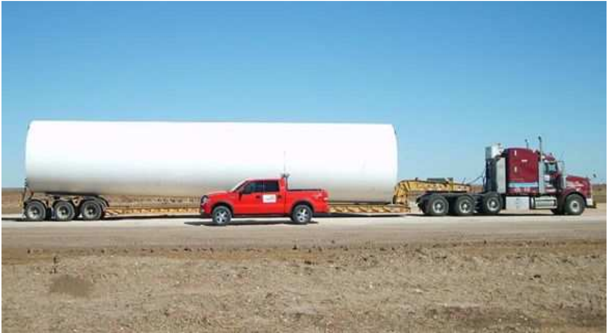
Photo 2: Tower Section transported on Lowbed Truck (routes with No height restrictions).
