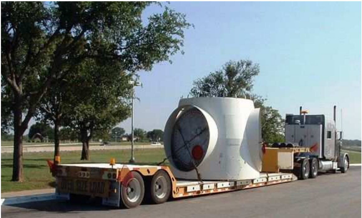
Photo 7 : Rotary Hub transported on special Lowbed. Note the limited ground clearance available.
