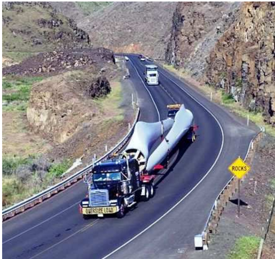
Photo 5 : Two WTG Blades transported simultaneously on one truck to reduce number of truck trips required. Special truck and support framework are required
