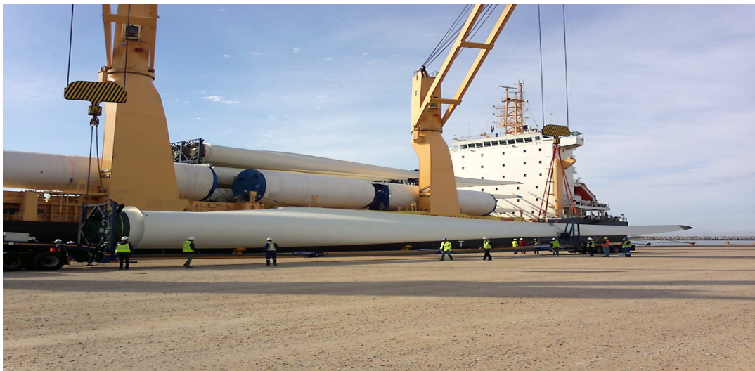
Photo 9 : Turbine shipping vessels equipped with on-board cranes
