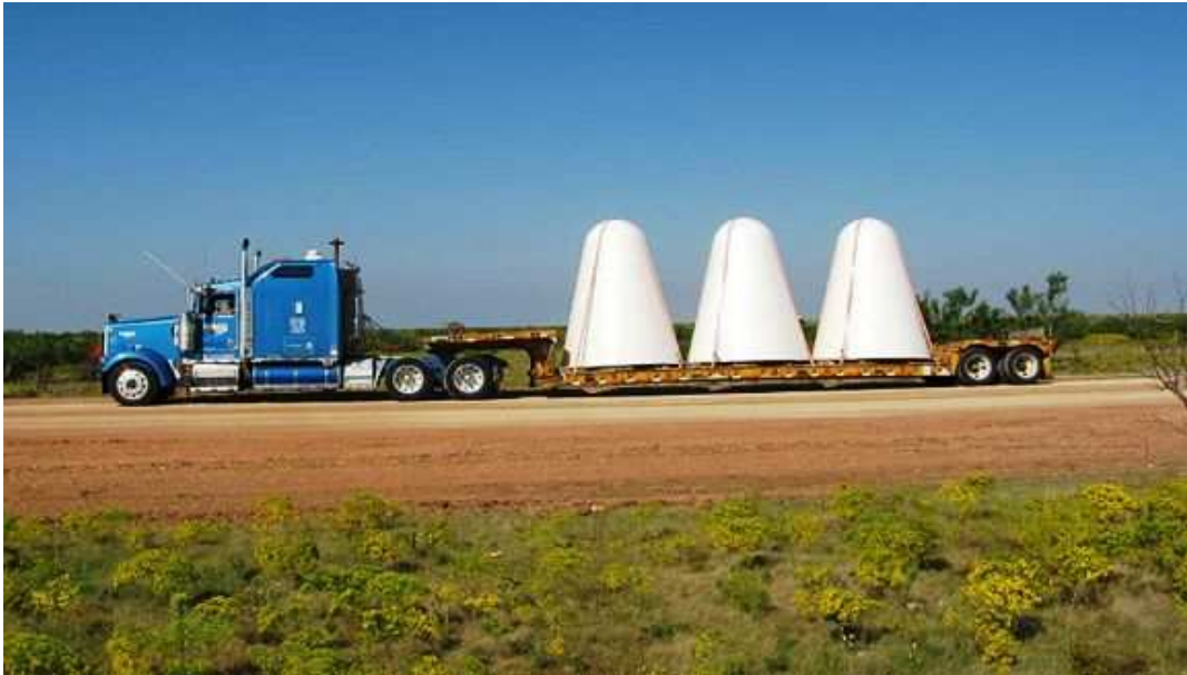
Photo 8 : Three (3) Rotary Hub nose units transported together. These smaller components are often transported with the Rotary Hub on a single truck.
