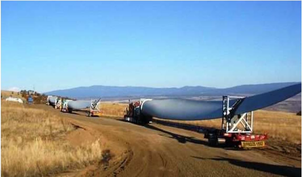
Photo 4 : WTG Blades transported with special "Centre Beam" Abnormal Long Trucks. Note special support frame for blade tips.
