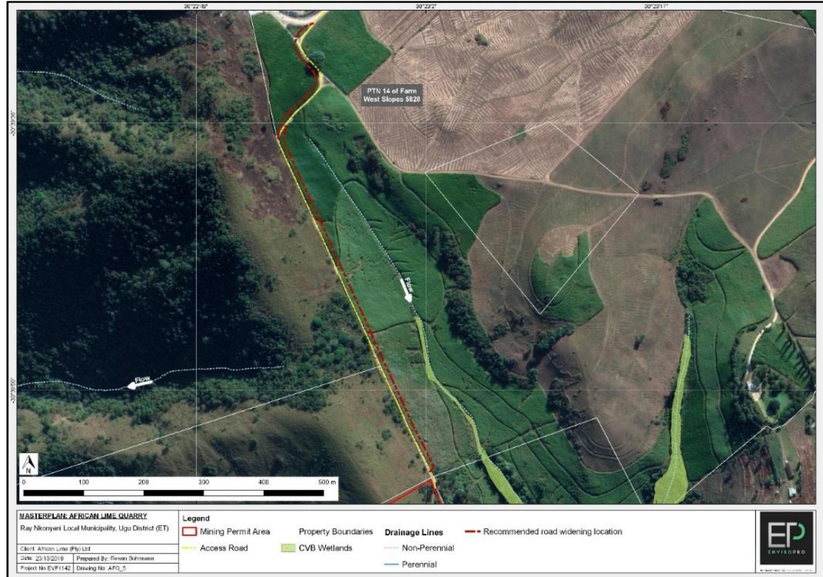
Figure 2: Red dash/ dotted line indicating the section of existing access road where widening is recommended (in the formally cultivated and degraded vegetation types).
