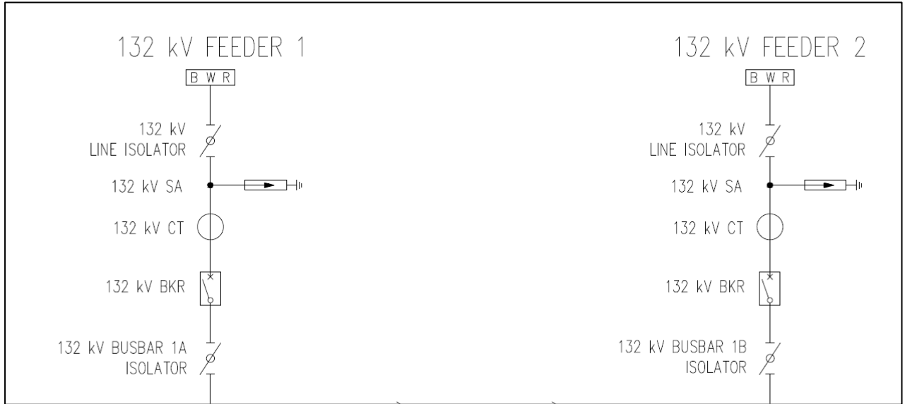
Figure 28: 2 x 132kV Incoming Feeder bays
