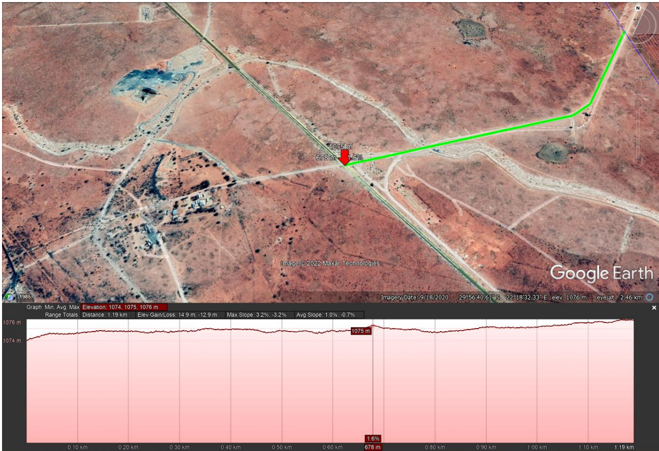
Figure 2-2: Horizontal Alignment (Source Google Earth)
