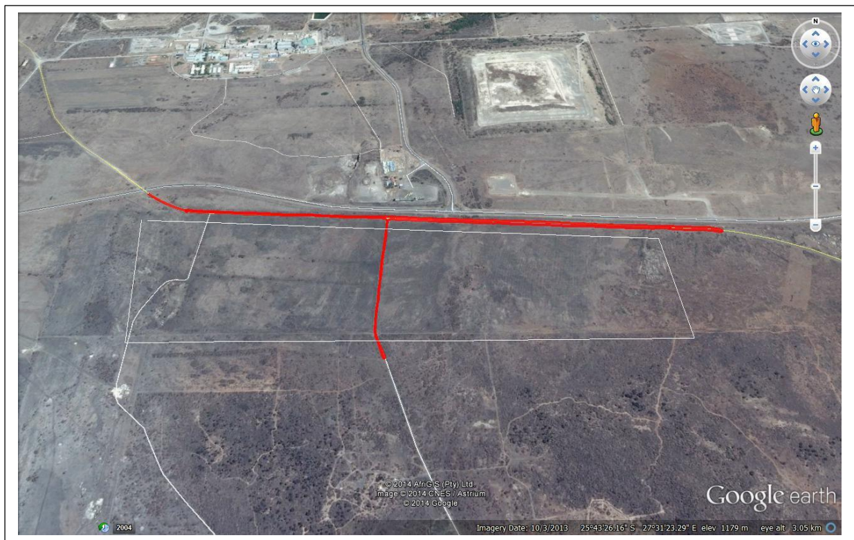
Figure 4- The main track of the field survey that was recorded with a mounted GPS instrument when surveying the Project Area. Pedestrian surveys were conducted in all directions from the main track. The largest part of the Project Area was utilized for cultivating crops such as maize in the past (above).
