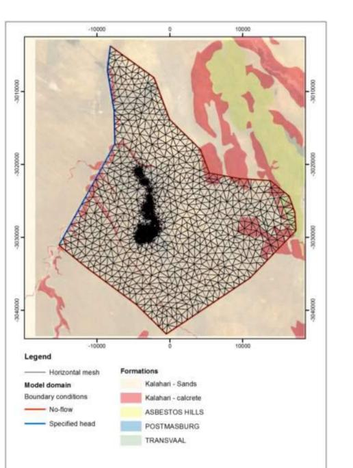
FIGURE 9-6: GROUNDWATER MODEL HORIZONTAL MESH
